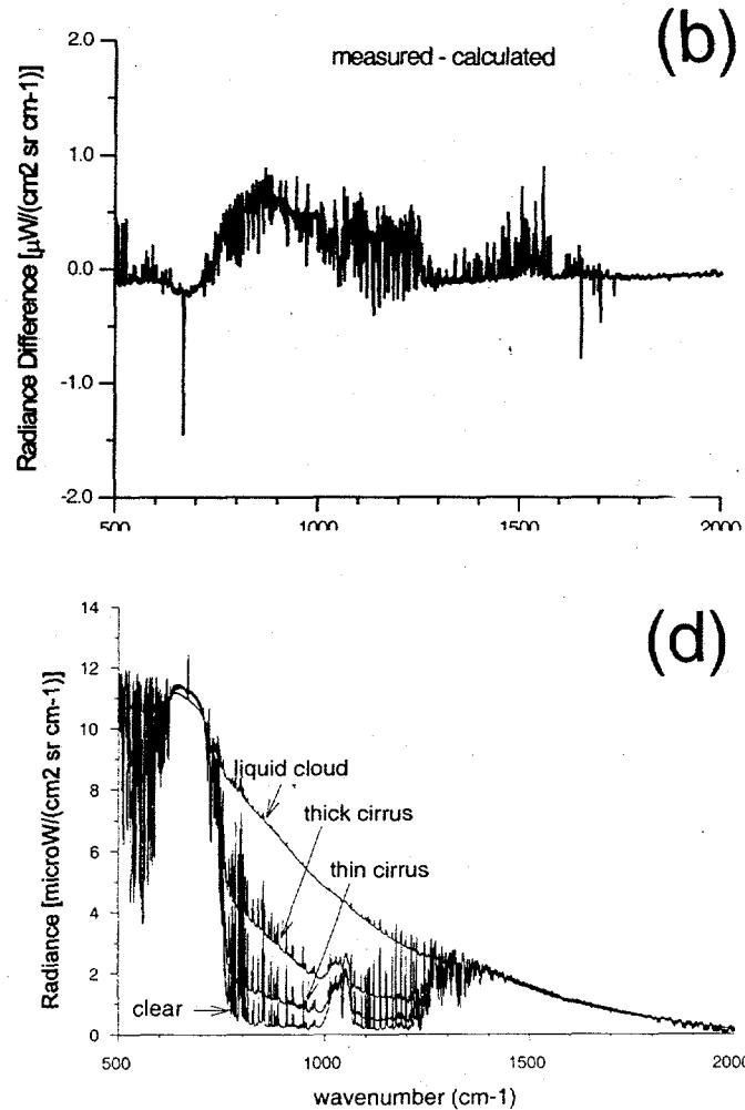
Figure 1. (a) FTIR measurement during clear conditions in Kavieng, Papua New Guinea; (b) difference between measured and calculated radiances; (c) FTIR measurements for various conditions in Kavieng, PNG; (d) FTIR measurements for various mid-latitude atmospheric conditions.
