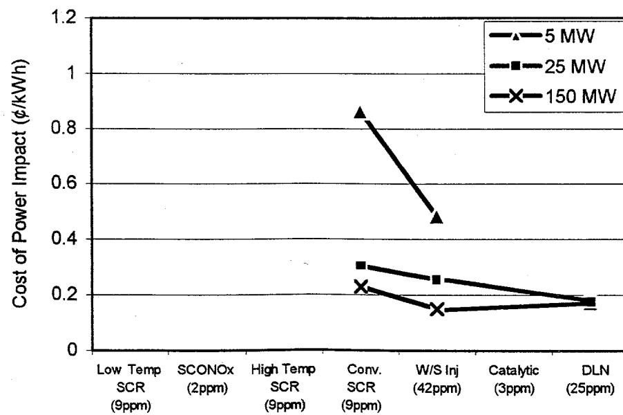
Figure S-2. 1993 EPA Comparison of NO<sub>x</sub> Control Technologies
