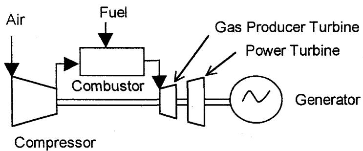
**Figure 2-1. Components of a Gas Turbine**
