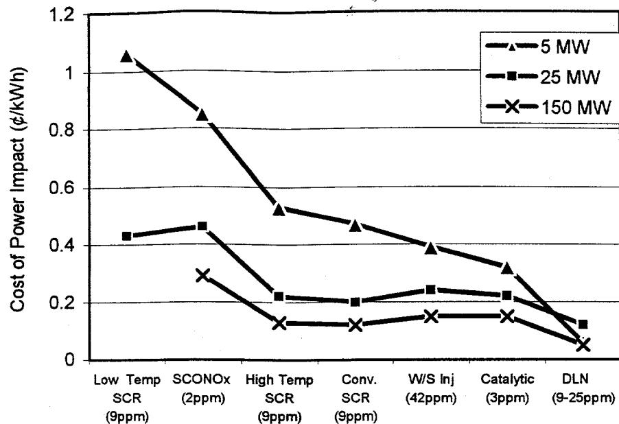
Figure S-1. Comparison of NO<sub>x</sub> Control Technologies (1999)
