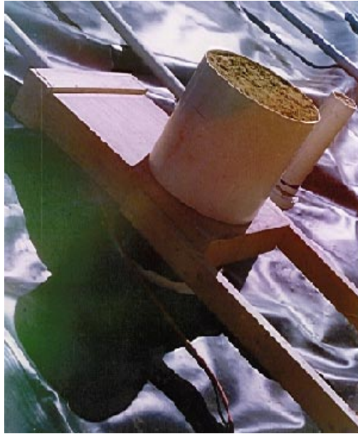
Figure 15. Photograph of engineered leak valve assemblies. Assembly in the foreground simulates a 15-in. diameter leak, in a 2 ft. thick barrier. Assembly in the background simulates a 4-in. diameter leak in a 2 ft. thick barrier.
