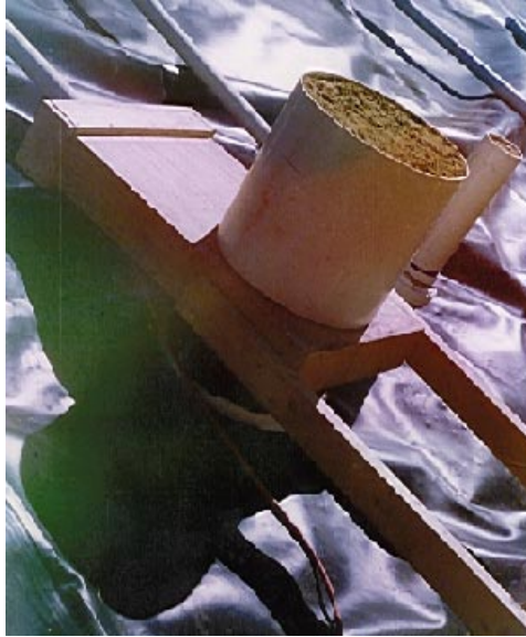
Figure E3. Photograph of engineered leak valve assemblies. Assembly in the foreground simulates a 15" diameter leak, in a 2' thick barrier. Assembly in the background simulates a 4" diameter leak in a 2' thick barrier.
