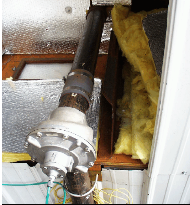
Figure 6. Goyen pulse valve and sight port at top of AHPC.
