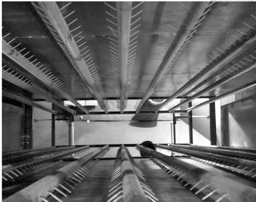
Figure 3. View from top of the AHPC with tube sheet and bags removed showing two rows of nine discharge electrodes.
