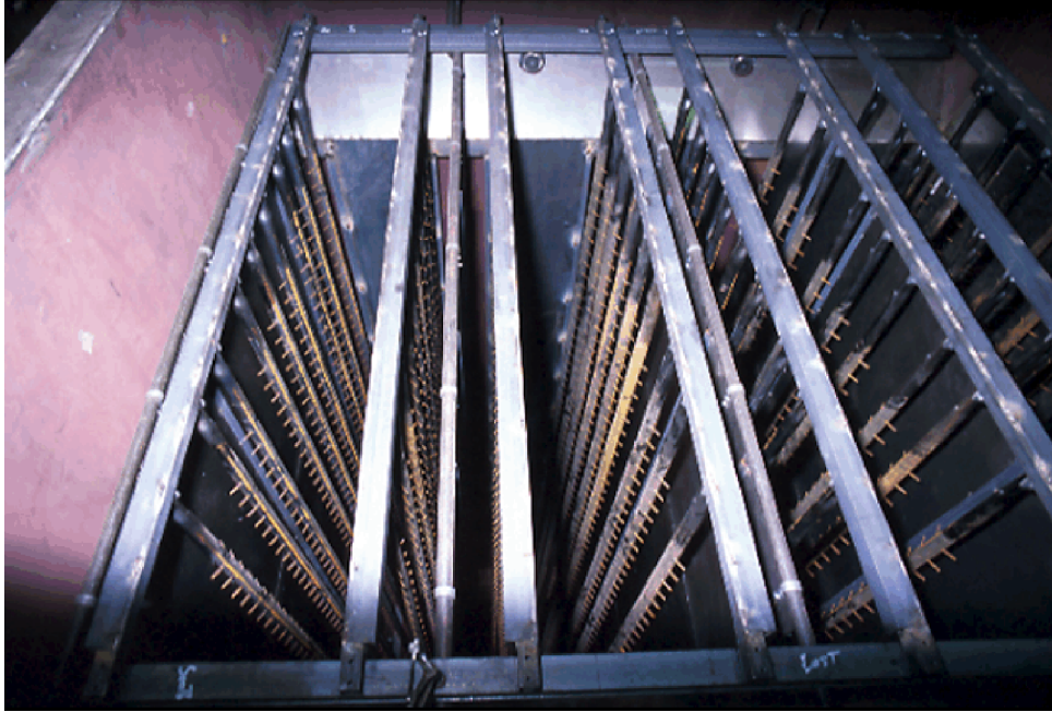
Figure 2. Internal arrangement of directional electrodes and plates shown without bags and tube sheet.
