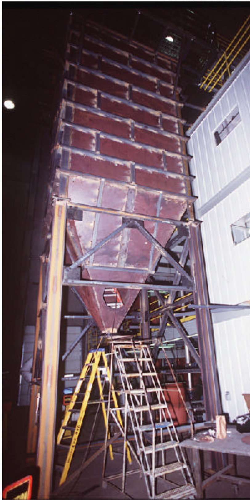
Figure 5. Erected AHPC vessel on support stand at the EERC.
