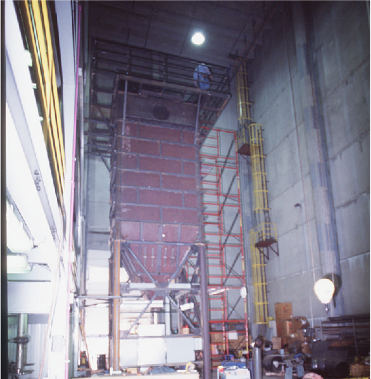
Figure 4. AHPC erected in the EERC high-bay pilot plant. Note that the top of the AHPC will have a walkway around all sides as shown here.
