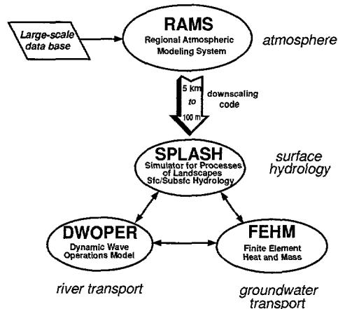
Figure 2. Schematic of the Los Alamos coupled modeling system to address water resources.
