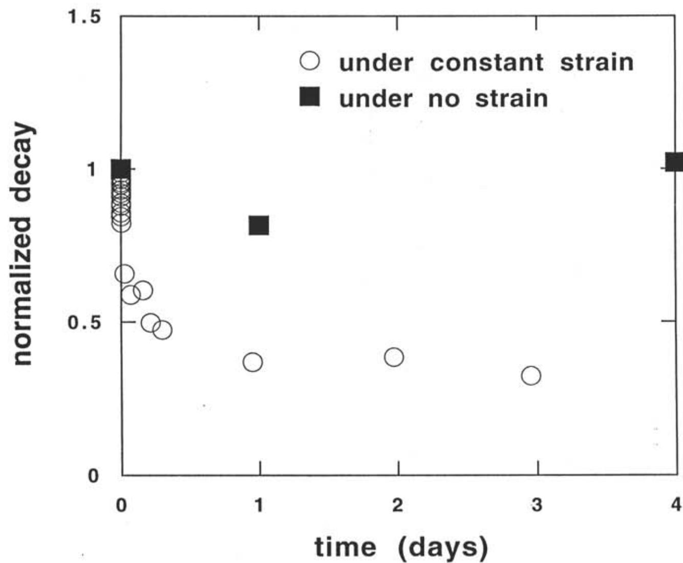
13. A dramatic difference in time scale is seen between the two tests and, and if one were not careful to perform both tests, different physical pictures could emerge. For example, if we only examined the change in total crosslink density as the sample ages by performing a simple "modulus" test, one might conclude that (a) not much chemistry actually takes place and (b) it happens fairly slowly (i.e. over a month or so).
