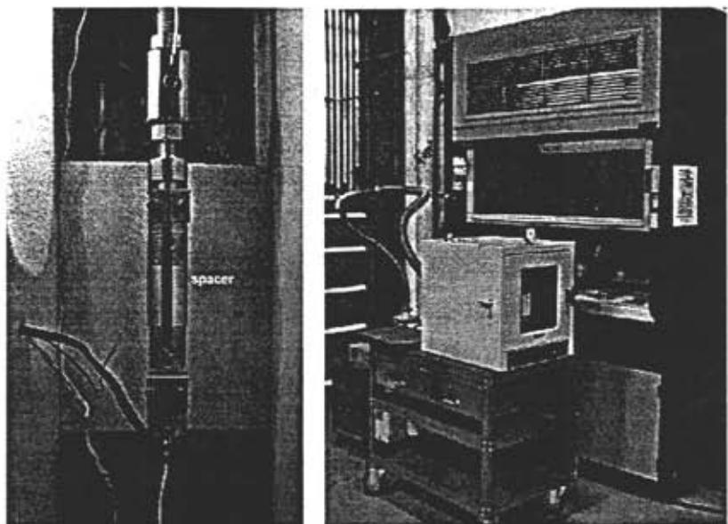
Step 7: The specimen-grips-spacer assembly is placed in a vacuum oven at elevated temperature.
