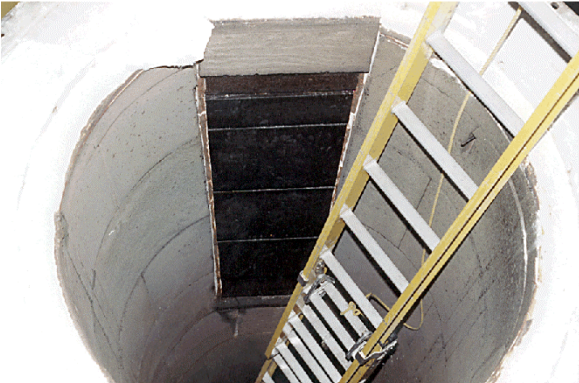
Exhibit 2.2-33 Photographs of the LRAH Panel Inside of the Slagging Furnace Following the January (top) and February (bottom) Tests
