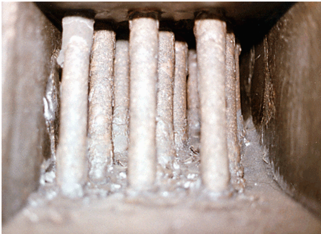
Exhibit 2.2-12 Photographs of Slag Screen Tubes Following the January (top) and February (bottom) Tests
