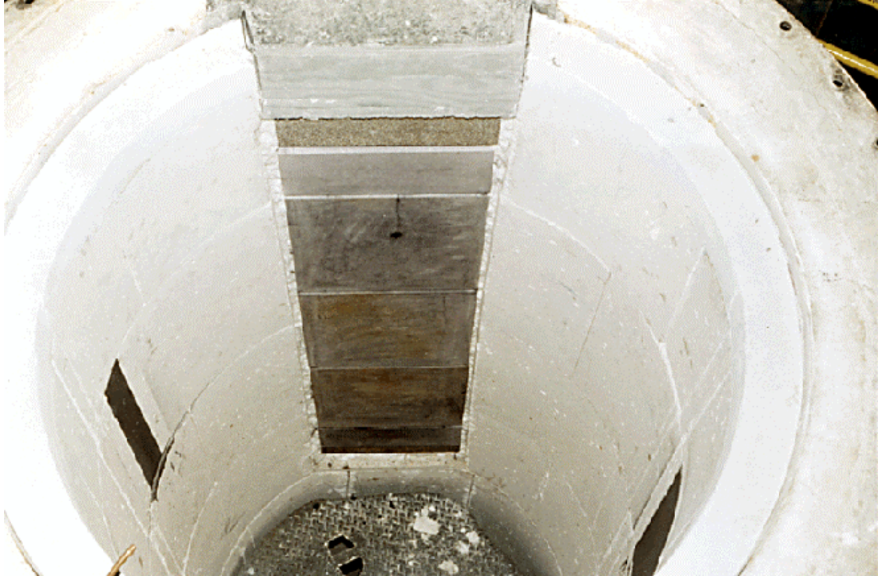
Exhibit 2.2-32 Photograph of New Ceramic Tiles on the LRAH Panel Inside of the Slagging Furnace Prior to the January Test
