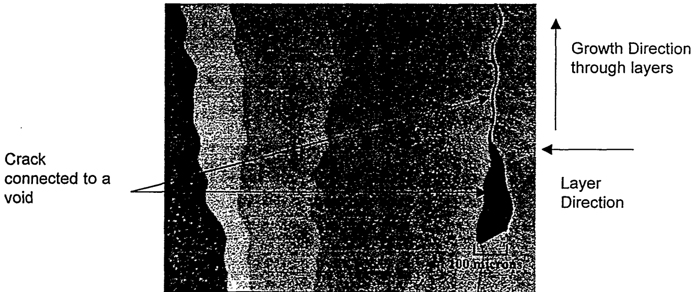
Figure 8. This tungsten microstructure, showing a large void and associated crack, was produced with the same parameters as the sample in Figure 7, except the power was lowered to 190w CW.
