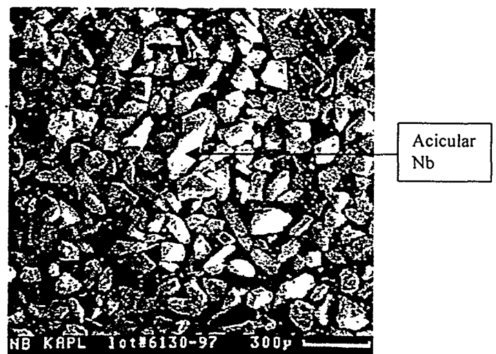
Figure 3. The SEM photograph shows niobium powder particles, (-200mesh), assumed to be made by electron beam melting, hydride de-hydride processing. Acicular shaped particles produced some nozzle clogging during DLF processing.
