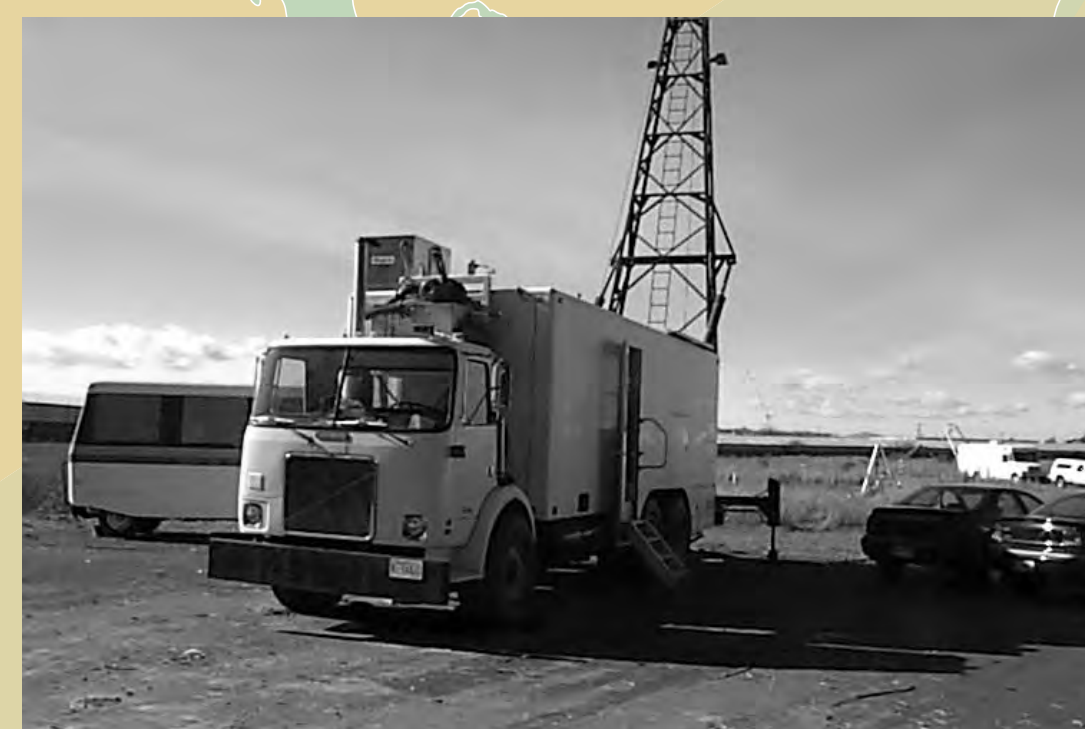
Logging mast fully extended on the LLNL receiver truck with the rear hydraulic stabilizer system activated. The large fuel capacity allows over 140 hours of operation in remote field sites. The transmitter truck is shown to the far right of the figure at the Richmond Field Station, California - a separation distance of 52 meters.
