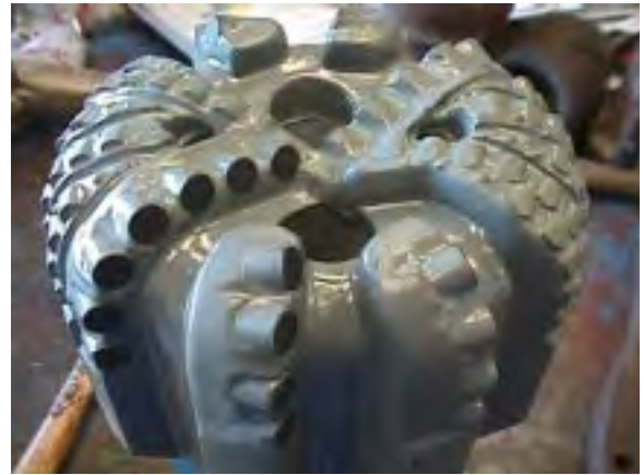
Fig. 14. DOE Hybrid TSP/PDC Bit
