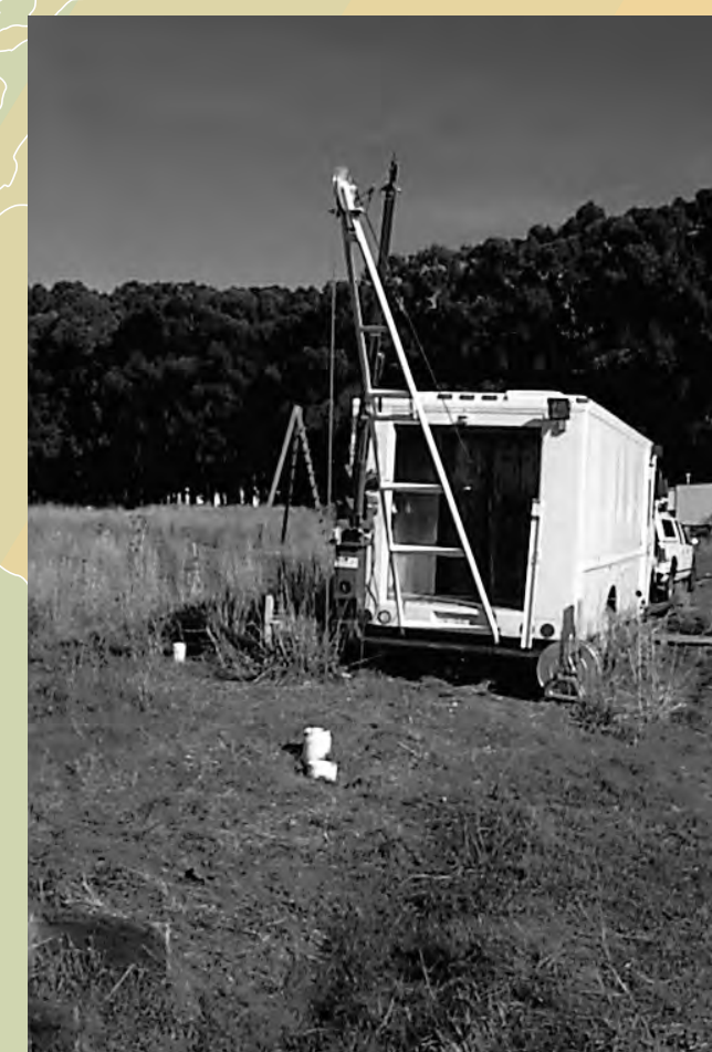
Rear view of the LLNL transmitter truck. The mast is controlled by a hydraulic boom for positioning over boreholes. The site is at the Richmond Field Station, California
