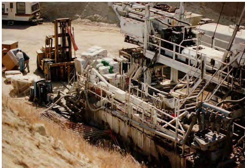
Fig. 20. Golden State Drilling Rig Mud System
