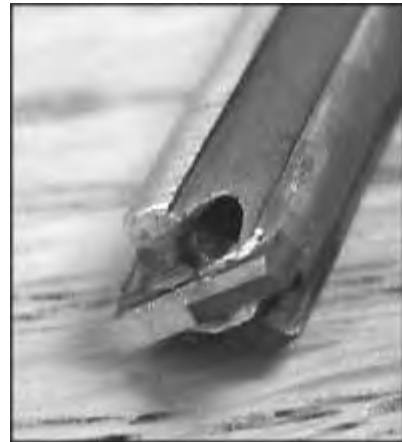
Figure 9. Mancos Shale drilling with backrake cutter at 60 rpm, 21 MPa ambient pressure.
