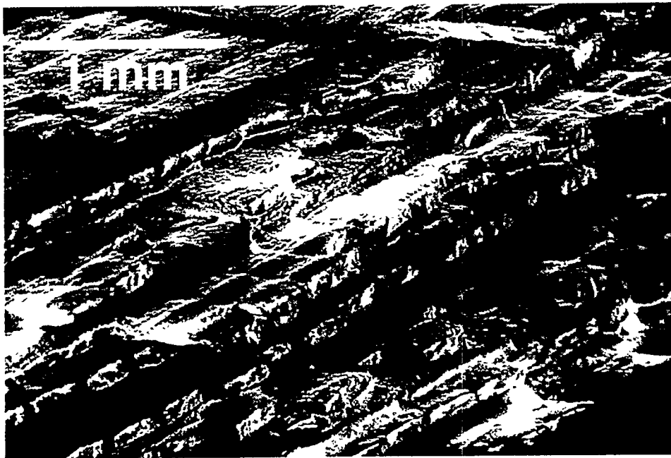
Figure 6. SEM photomicrograph of tensile fracture surface of ±45° Si 3 N 4 /BN FM tested in biaxial mode; interlayer delamination is evident
