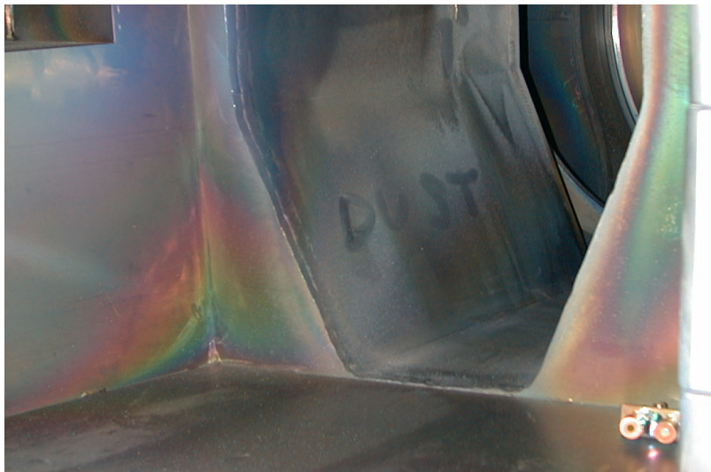
Figure 2.18. Photograph showing dust collected on the surfaces of a penetration port.
