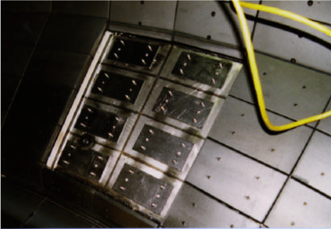
Figure 2.5. Photograph of the lower baffle with the 337 – 345° tiles removed.
