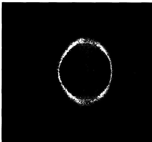
Figure 2. Three-dimensional visualization of the output from the LINAC3D code showing the particle density in a mismatched beam in the presence of nonlinear accelerating fields. The beam is moving from left to right, and the left-right asymmetry is due to the nonlinearities. The diffuse region far from the central core constitutes the beam halo. Understanding and predicting beam halo is a major issue in next-generation high-current linear accelerators.
