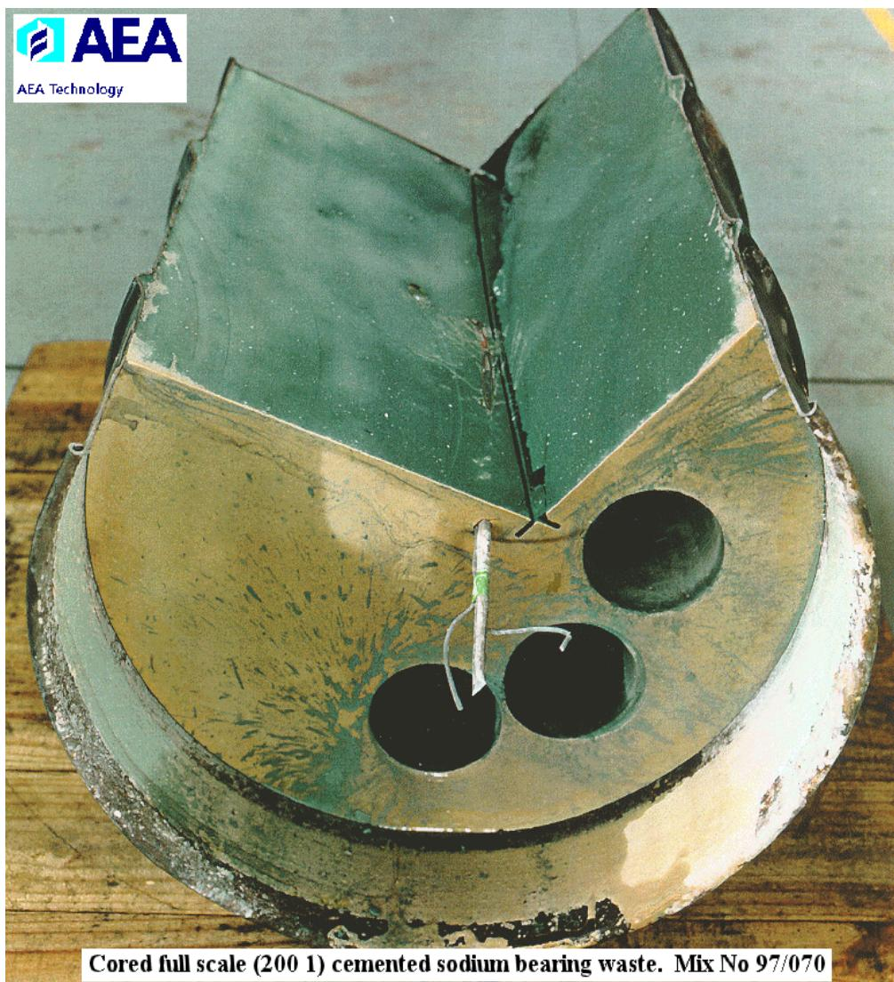
**Figure 2.** Cored full-scale (200 L) cemented sodium-bearing waste.
