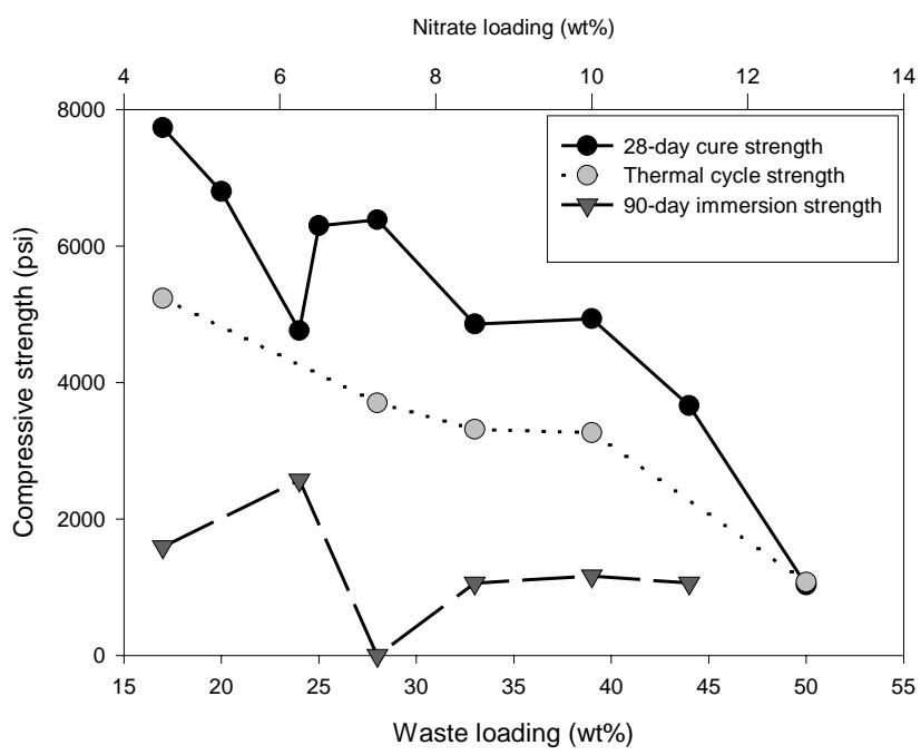
**Figure 1.** Influence of waste loading on compressive strength
