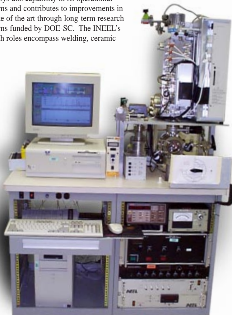
FIGURE 10. The secondary ion mass spectroscopy system concept was developed under a DOE-Basic Energy Science project. The system is used to detect very low levels of nonvolatile chemicals on surfaces.
