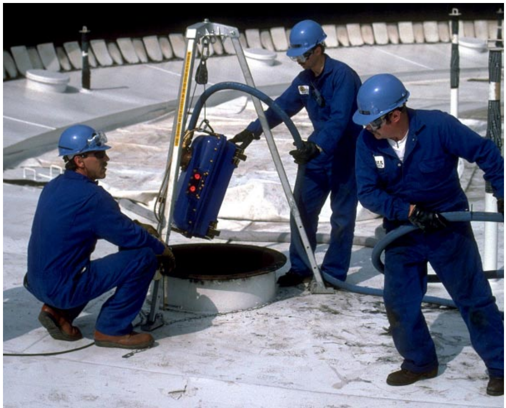
FIGURE 15. INEEL technologies improve fuel storage. The above picture shows the Maverick Tank Inspection Robot (initially developed at the INEEL) being lowered into a tank of diesel fuel to inspect the integrity of the tank floor. Automated equipment allows these inspections to be performed with little or no risk to operators and the environment.
