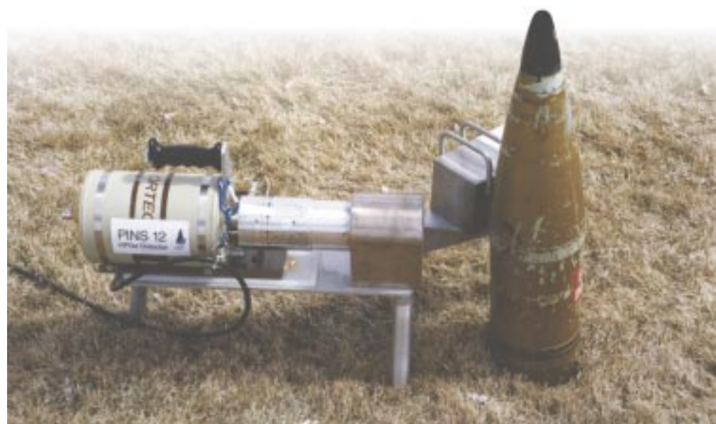
FIGURE 8. The portable isotopic neutron spectroscopy system received an R&D 100 Award in 1993. The INEEL developed the system as part of a DOE NN-20 project to support chemical weapons treaty verification. The U.S. Army routinely uses this system to nonintrusively and safely identify the contents of suspect chemical warfare munitions and containers.
