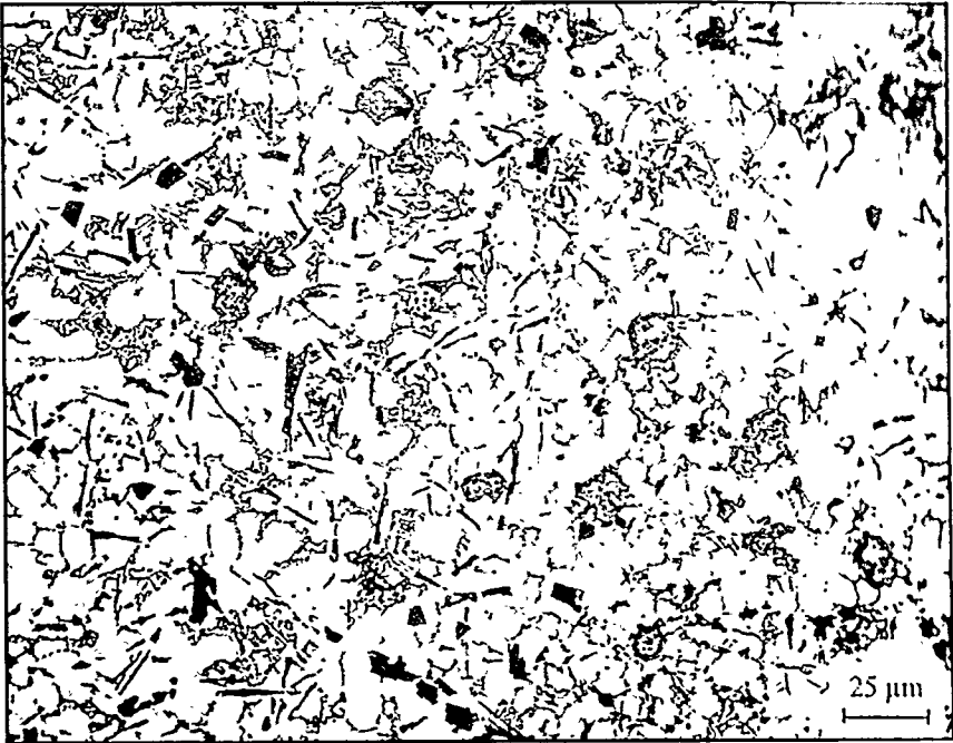
Fig. 3.24.5. Representative optical micrograph of Alloy 24, as die cast condition (400X).
