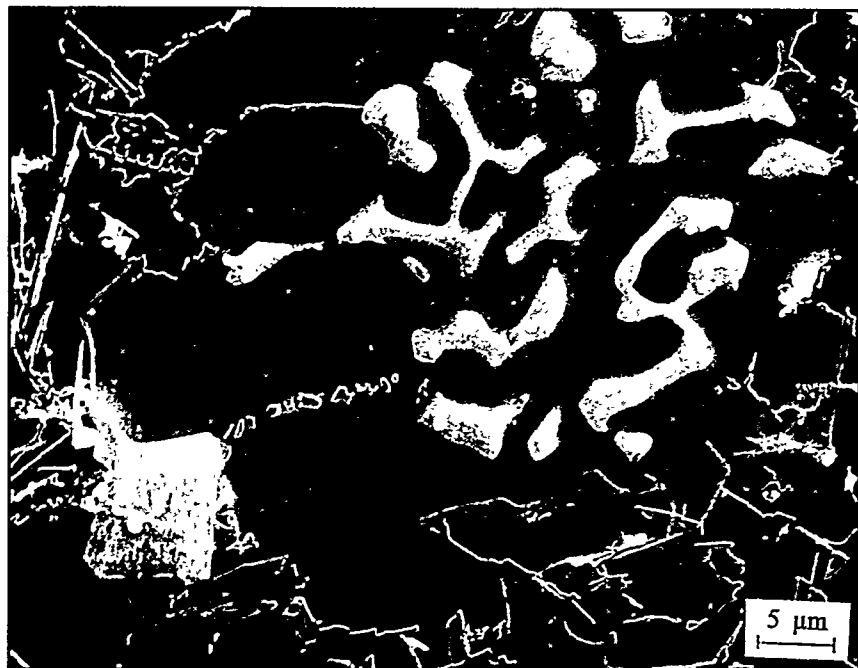
Fig. 3.21.7. SEM micrograph of Alloy 21 in the die cast condition, showing Fe bearing Chinese script, polyhedral crystals and needles, and the Al-Si eutectic structure (2000X).
