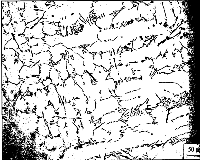
Fig. 4.1.2 (b) Graphite mold casting (cooling rate: \sim 750^\circ\text{C}/\text{min} ). The above photographs are microstructures of Alloy 1 (7.15%Si, 0.01%Mg, 0.68%Fe, 1.24%Cu, 0.01%Ni, 0.01%Cr, 0.01%Mn, 0.01%Ti, 0.44%Zn and 0.00%Sr) solidified at different cooling rates.
