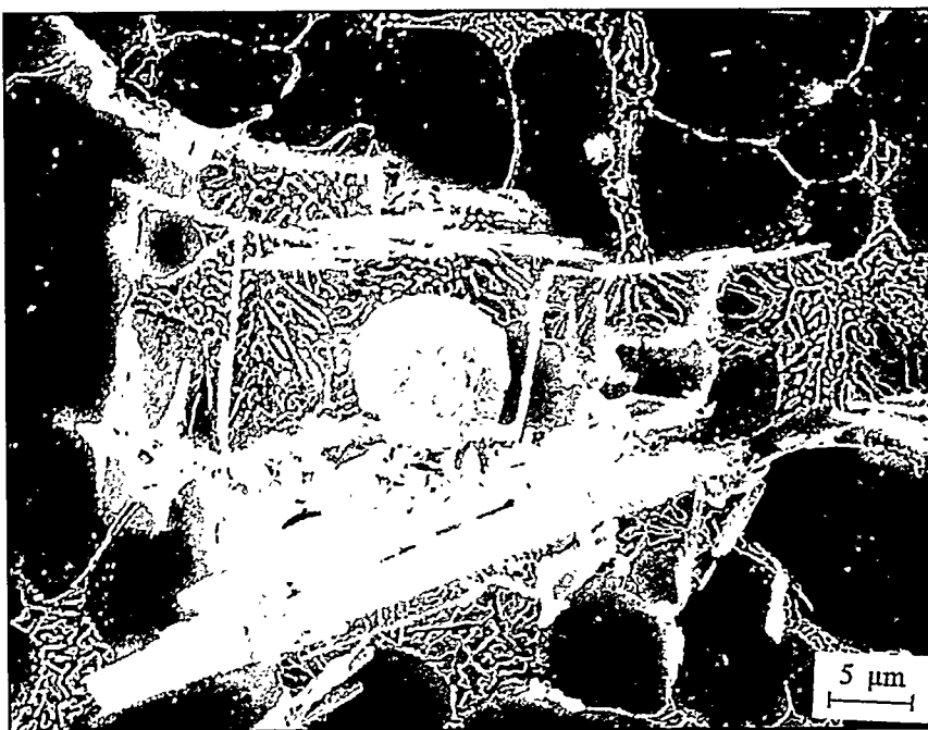
Fig. 3.7.7. SEM micrograph of Alloy 7 in the die cast condition, showing large Fe bearing needles, Cu bearing particles, and the Al-Si eutectic structure (2000X).
