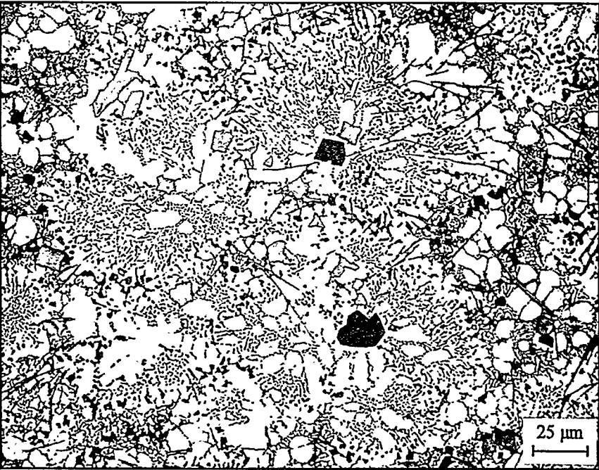
Fig. 3.12.5. Representative optical micrograph of Alloy 12, as die cast condition (400X).
