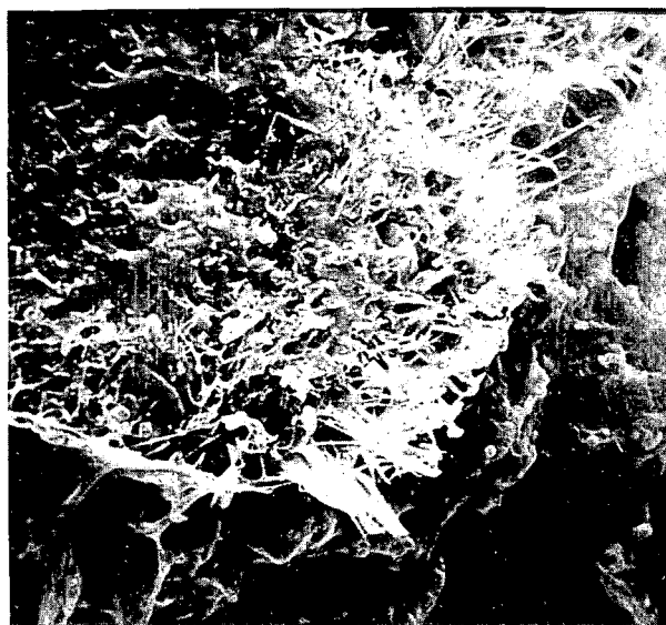
Fig. 4 SEM photograph of very fine illite hairs in pore space. 1000X.
