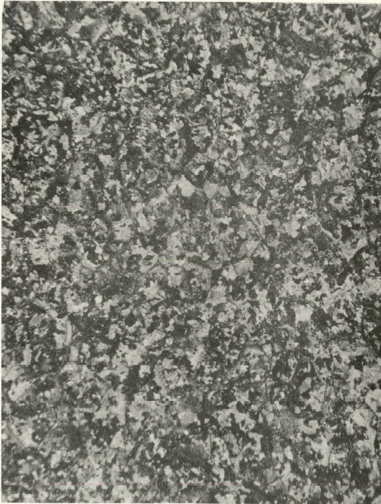
L383-2 Figure 2. OVERAGED URANIUM-2 WEIGHT PERCENT MOLYBDENUM ALLOY. (Bright Field Illumination; 100X)
