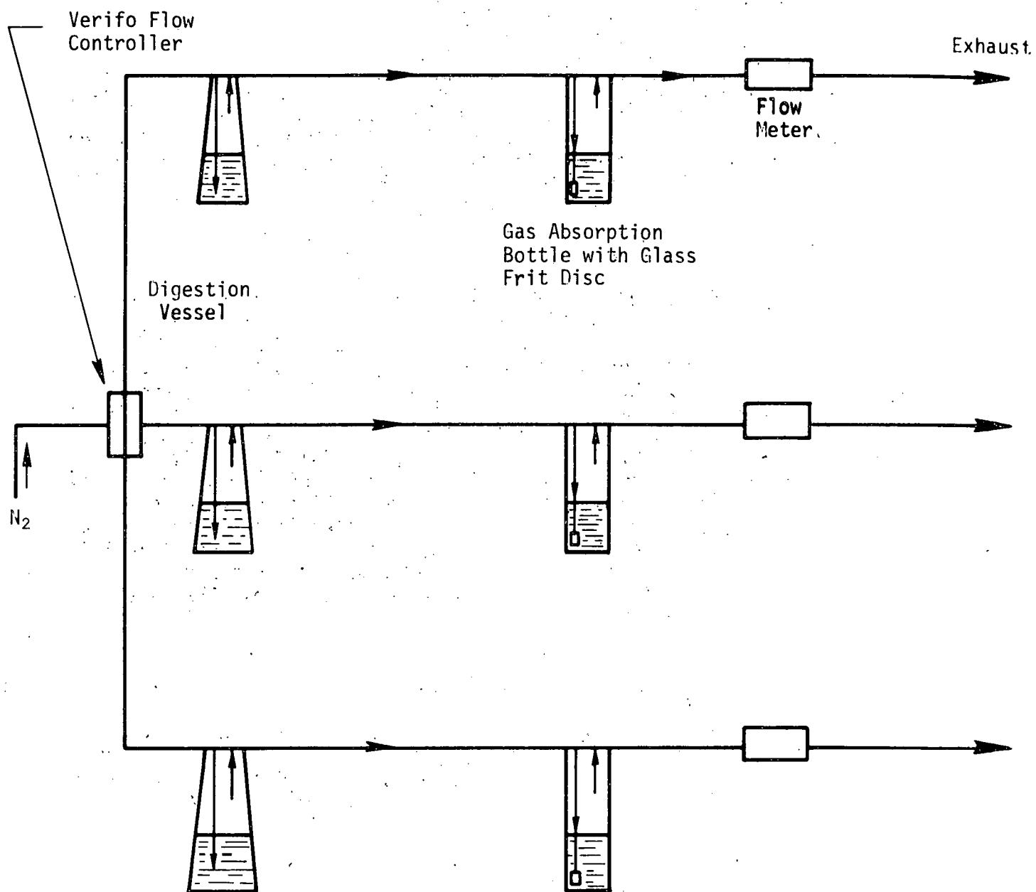
Fig. 1. Gas Train for Inorganic Chloride Analysis
