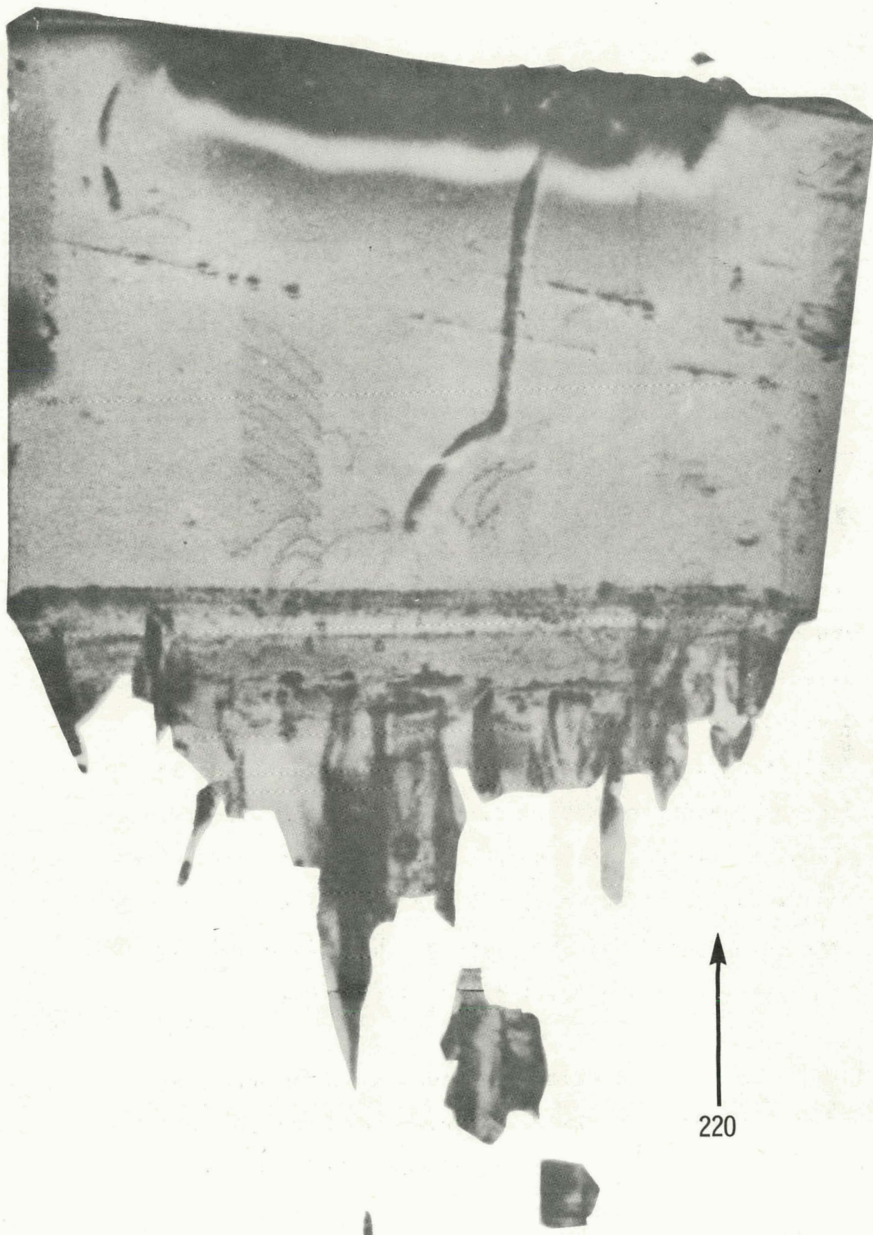
Fig. 11. An x-ray topograph of a typical crystal-seed interface showing the catastrophic collapse of seed orientation due to heavy twinning.
