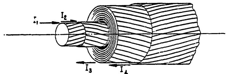
Fig. 2. Magnetic fields on inner conductor tape segments.
