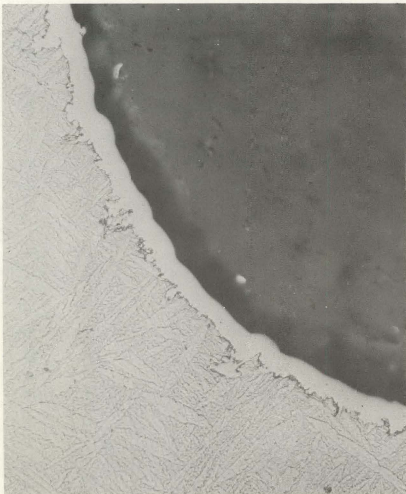
MS-75-0115-5 Figure 9. PHOTOMICROGRAPH OF URANIUM-0.75 TITANIUM ALLOY AFTER ELECTRICAL DISCHARGE MACHINING, WIRE BRUSHING, AND NICKEL PLATING. (Bright Field Illumination; 400X)
