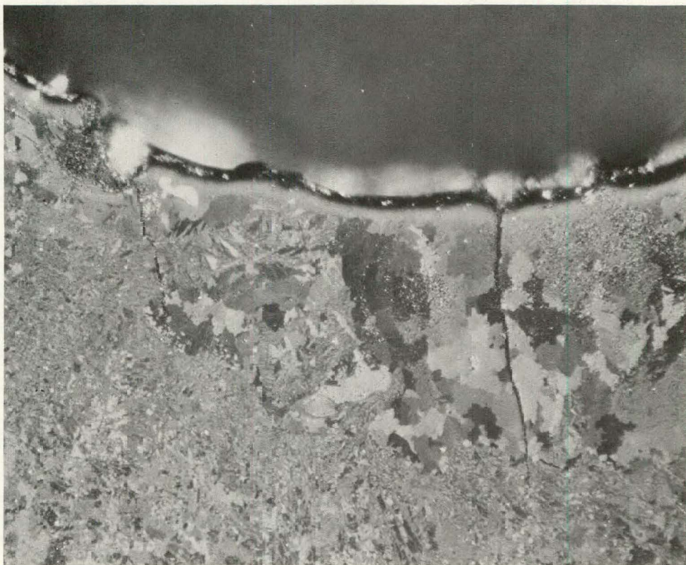
Figure 2. PHOTOMICROGRAPH OF URANIUM-0.75 TITANIUM ALLOY AFTER ELECTRICAL DISCHARGE MACHINING BY THE TEST 1 PARAMETERS OF TABLE 1. (Polarized Light; 250X)
