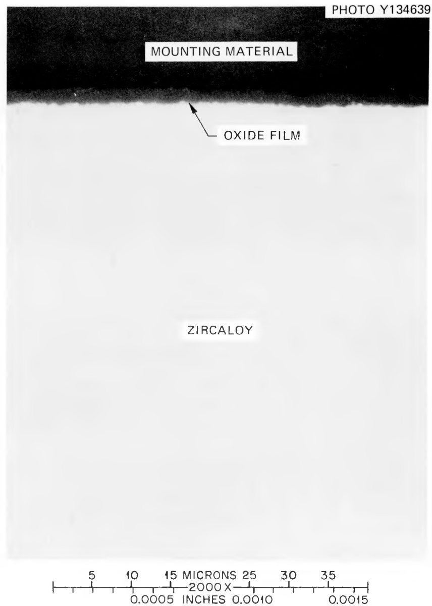
Fig. 3.5. Photomicrograph showing oxide film produced on tube 645 during oxidation run 4 (as polished; 2000X).
