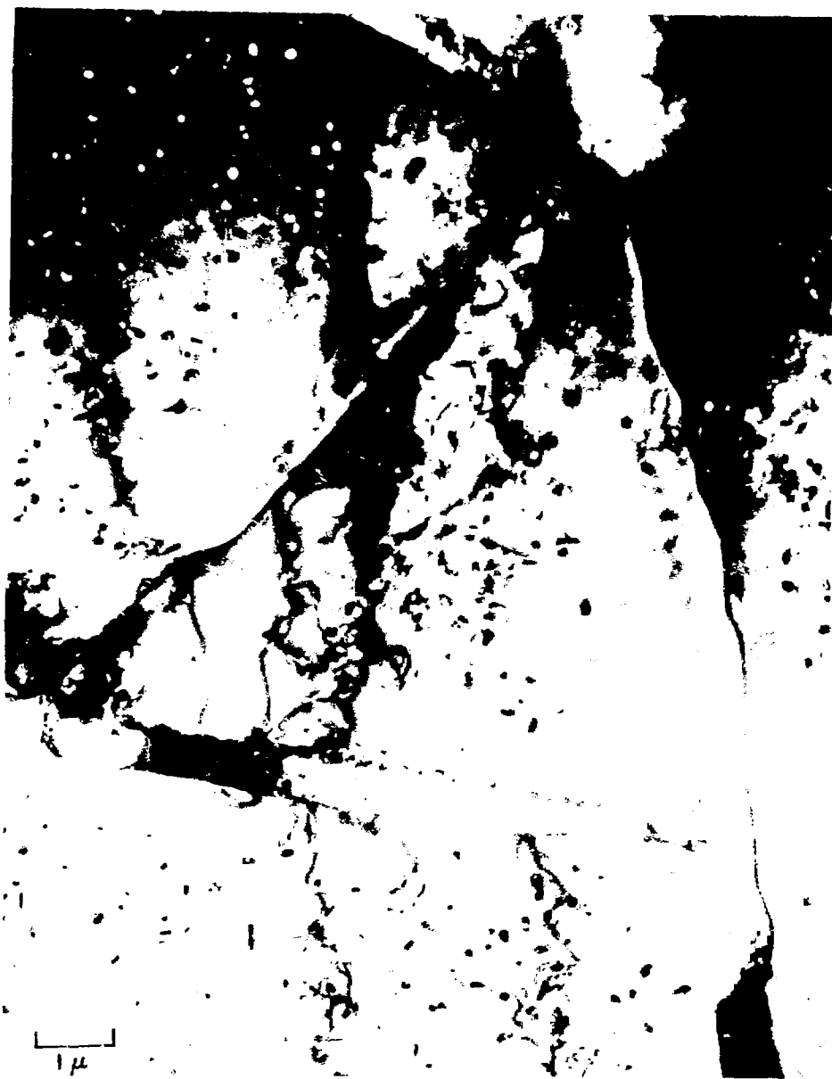
Fig. 11. Void and Precipitate Denuding Near Grain Boundaries in Vanadium Irradiated as Annealed at 650°C with 18 MeV Cu Ions to 5 dpa.
