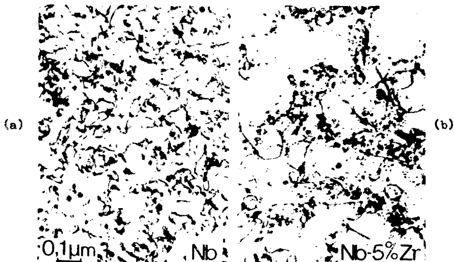
Fig. 5. Dislocation distributions in 1600°C heat treated commercial niobium and niobium - 5% zirconium irradiated to 3.6 \times 10^{22} fast neutrons/cm 2 at 600°C.
