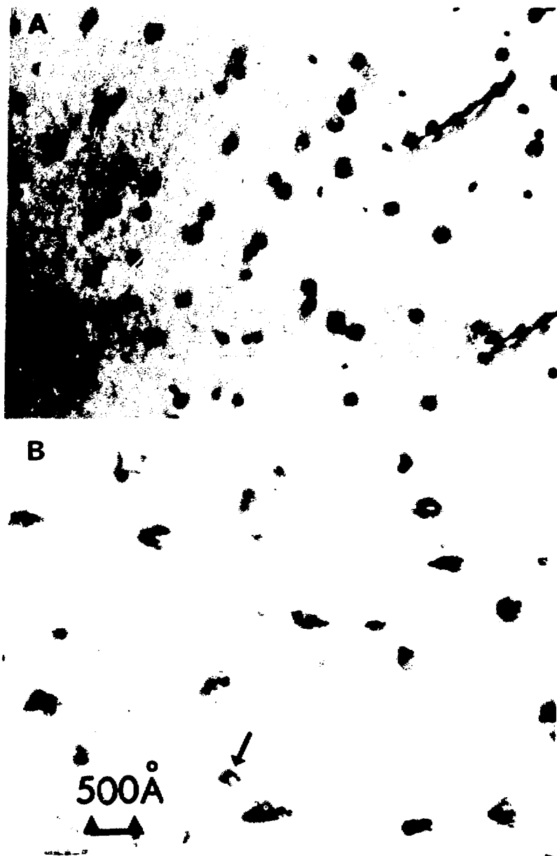
Figure 1 Comparison of damage structure in ST 316 steel after helium implantation (a) Small interstitial Frank loops formed after a 9 hour anneal at 600°C following 100 appm helium injection (b) Dislocation loop defects on which precipitates and helium bubbles nucleate during implantation with 100 appm helium at 600°C. (Arrow indicates large bubbles).
