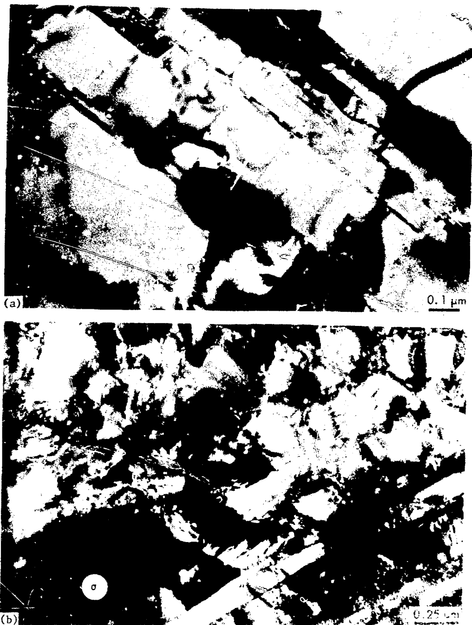
Fig. 5. Type 316 Stainless Steel, 20% Cold Worked, Irradiated at 550°C to 42 dpa and 2990 appm He. (a) Cavities in the matrix; (b) cavities at the grain boundary. Note \sigma -phase particle labeled \sigma .
