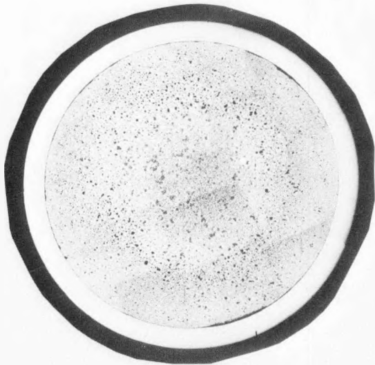
Fig. B.38. Cross Section of Element E-18, Subassembly C-2236S: 1 in. from Bottom of Fuel; ~6 at. % Burnup. As polished. Mag. 15X. Neg. No. MSD-163602.
