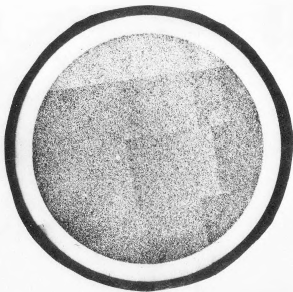
Fig. B.38. Cross Section of Element E-18, Subassembly C-2236S: 1 in. from Bottom of Fuel; ~6 at. % Burnup. As polished. Mag. 15X. Neg. No. MSD-163602.
