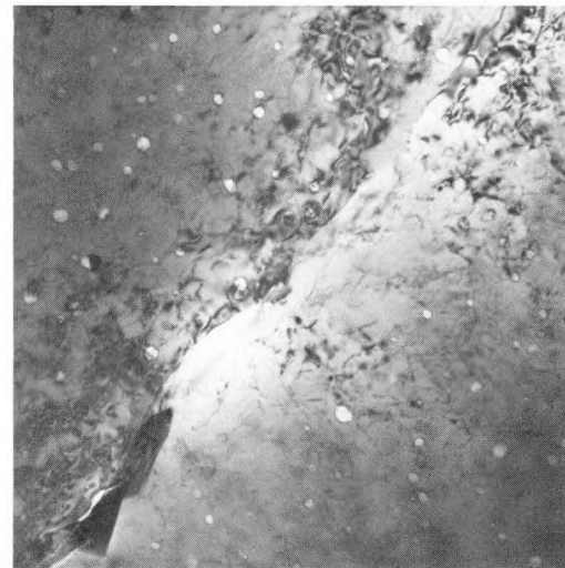
Fig. 29. TEM Micrographs of Types 304L (top) and 316 Stainless Steel (bottom) Mark-II Cladding, Showing Voids and Precipitates. Mag. 27,000X.
