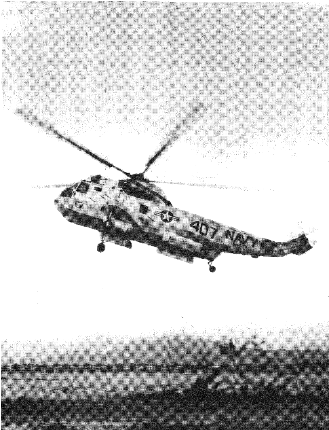
Figure 5. The Navy SH-3 equipped with gamma pods (front) and neutron detector pods (rear).
