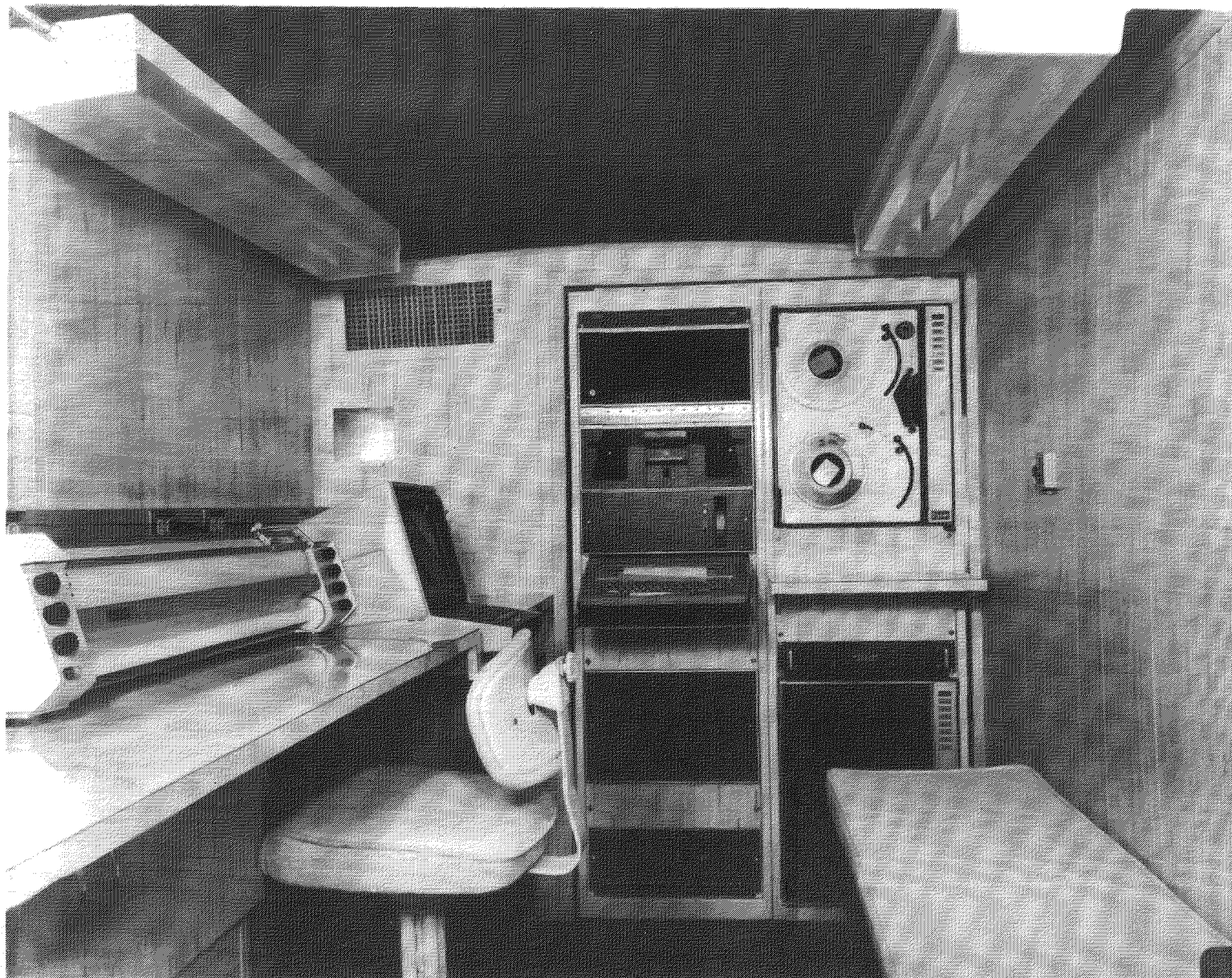
Figure 8. The REDAC (Radiation and Environmental Data Analyzer and Computer) mounted in a mobile van truck.
