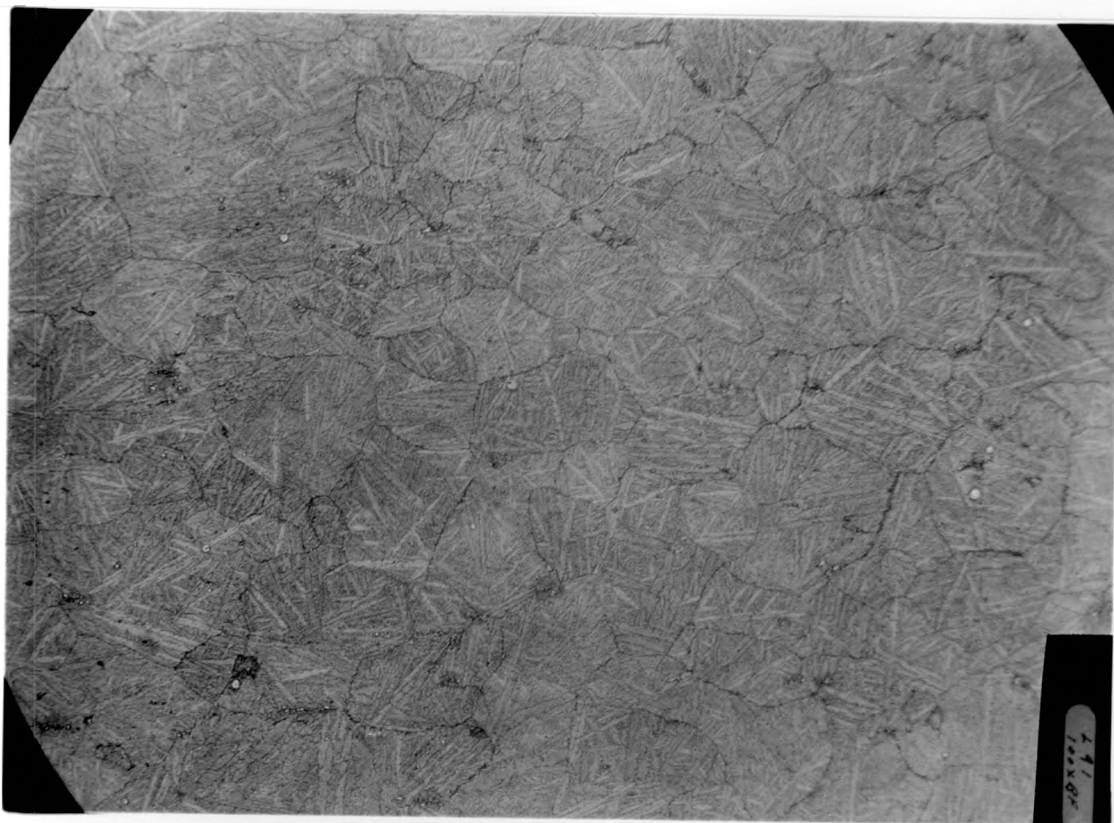
Figure 3. URANIUM-0.75 WEIGHT PERCENT TITANIUM WORKED AT 575°C (SMALL GRAINS) AND 630°C (LARGE GRAINS) AND SOLUTION TREATED AT 800°C
