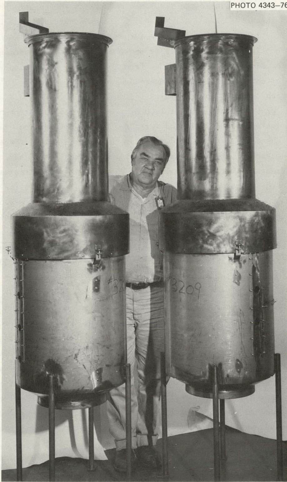
Fig. 13. Cooler housings for corrosion loop FCL-3.
