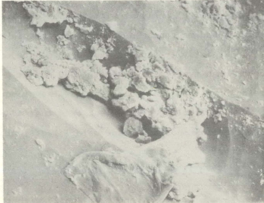
FIGURE 2. Run. 25. Seed/ingot interface at 2200X magnification showing inclusions.
