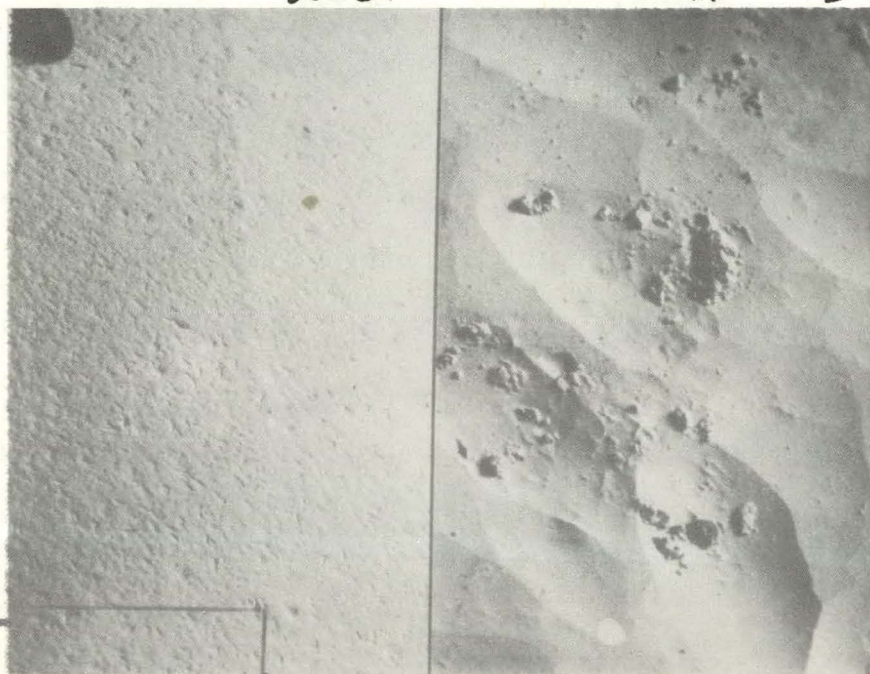
FIGURE 1. Run 25. Seed/ingot interface at 17X and 900X magnification.
