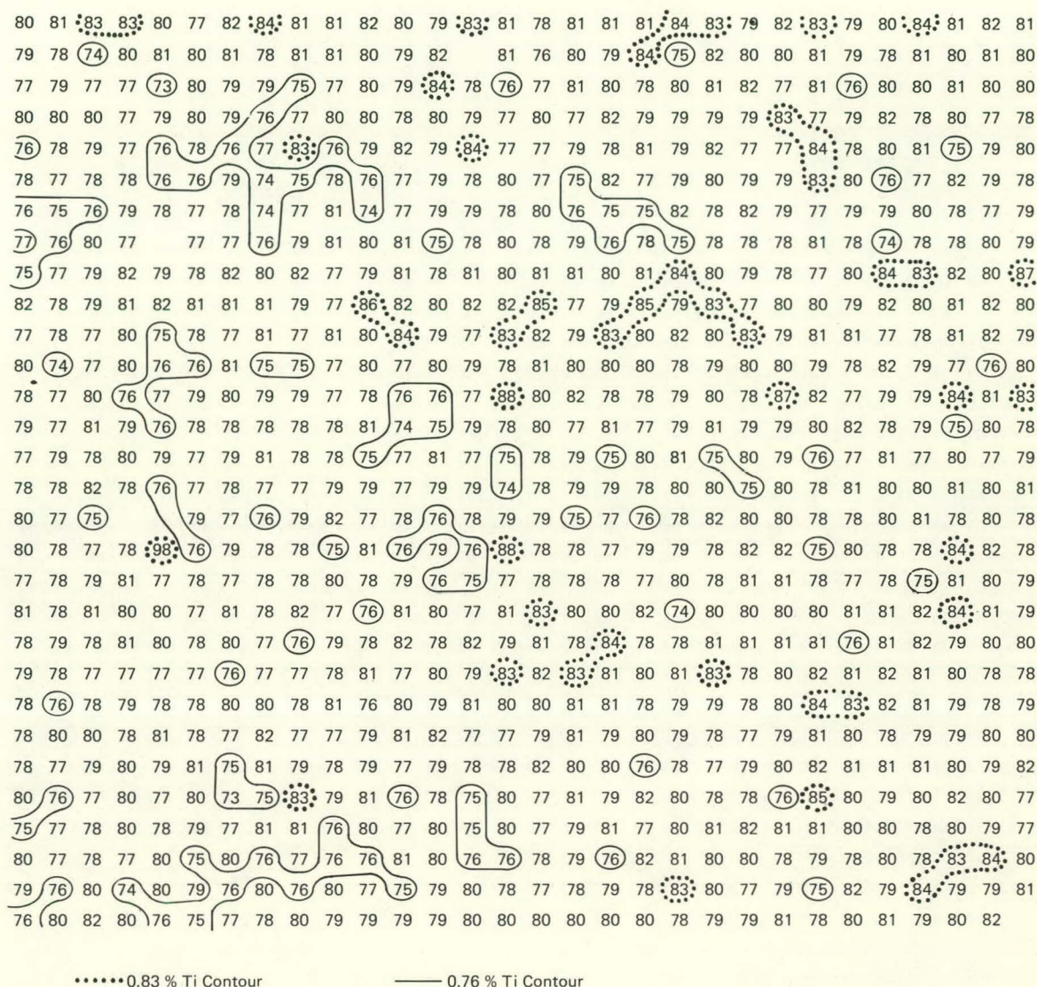
Figure 6. MICROSEGREGATION IN A URANIUM-0.75 TITANIUM CASTING AFTER ONE HOUR AT 800° C IN VACUUM AND WATER QUENCHED. (Data Points are about 4.5 \mu m Apart; Numbers are 10^{-2} % Titanium)
