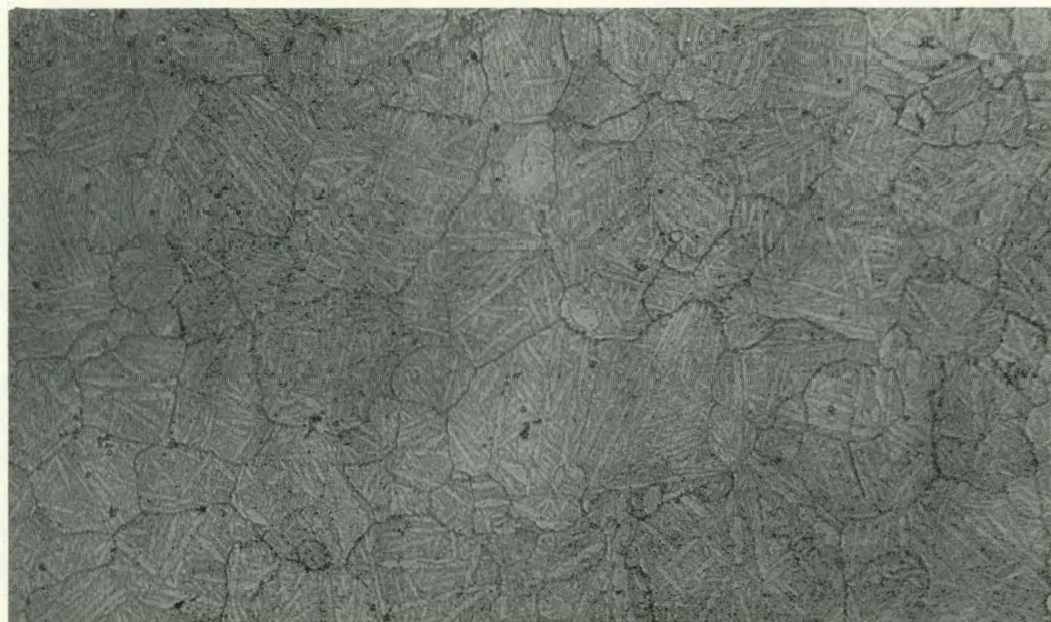
Figure 25. URANIUM-0.73 TITANIUM ALLOY THAT WAS HOMOGENIZED IN VACUUM AT 1000° C FOR 24 HOURS, HOT AND WARM ROLLED TO 30% REDUCTION, SOLUTION TREATED IN VACUUM FOR ONE HOUR AT 800° C, AND AGED FOR SIX HOURS AT 380° C. (Etched; Bright Field Illumination; 100X)
