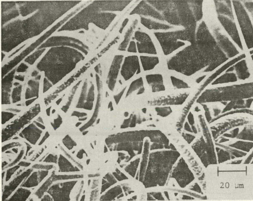
Figure 2-14. SEM Photograph of CVD Si Deposit on OI Glass GS211 at ~850°C in H 2 Atmosphere
