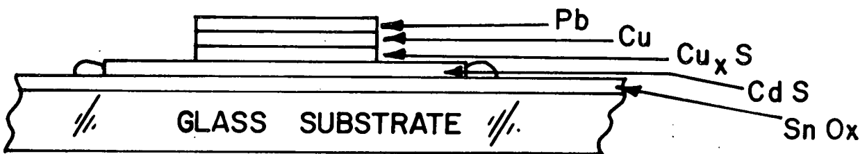
TEST CELL STRUCTURE BEFORE AND AFTER ETCHING AWAY OF PERIPHERAL Cu_x S
