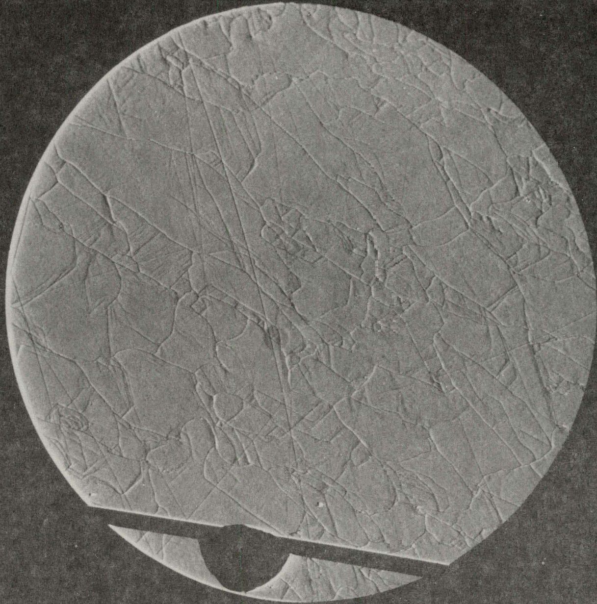
EBIC picture of sample area in lower right hand portion of wafer in previous figure.
