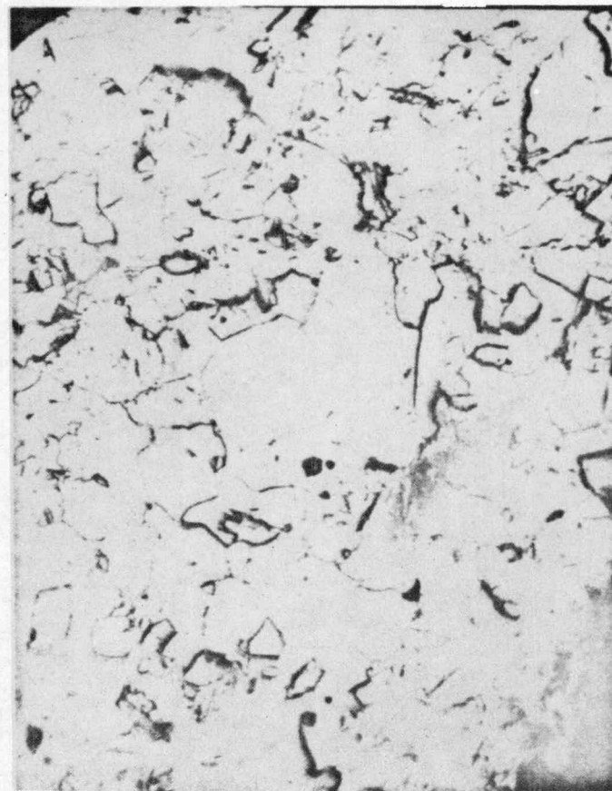
After Cycling- 100 cycles 520-1350°C (30 min per cycle) 75 cycles 630°C - 1385°C (30 min per cycle)
