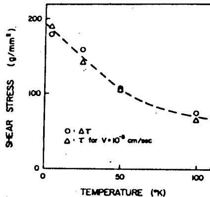
Fig. 3 - The increase of yield stress due to irradiation and the stress required to maintain the dislocation velocity at  $10^{-3}$  cm/sec are plotted against temperature.
