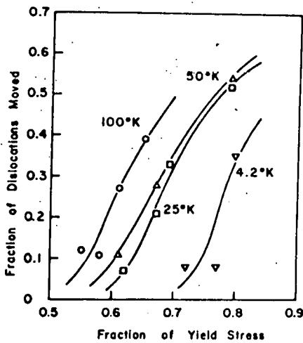
Fig. 2 - The fraction of dislocations moved as a function of applied stress. The applied stresses are normalized with respect to the yield stress of the corresponding temperature.
