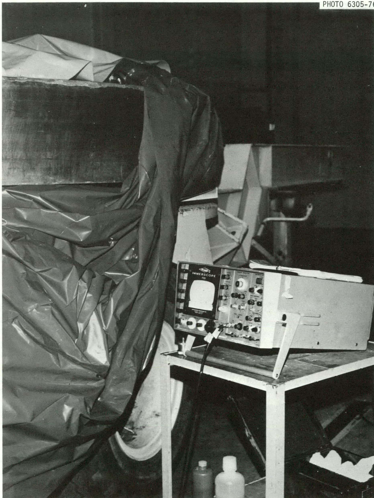
Figure 17. The Ultrasonic Testing of the Reactor Vessel Head After It Was Placed on the Truck for Storage
