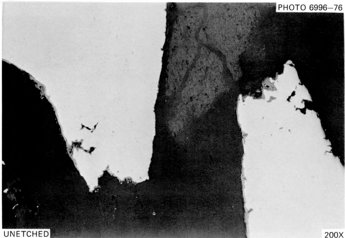
Fig. 3.10. Magnified (and inverted) view of crack in groove 3 of fuel simulator 2828016. (Original reduced 5%)
