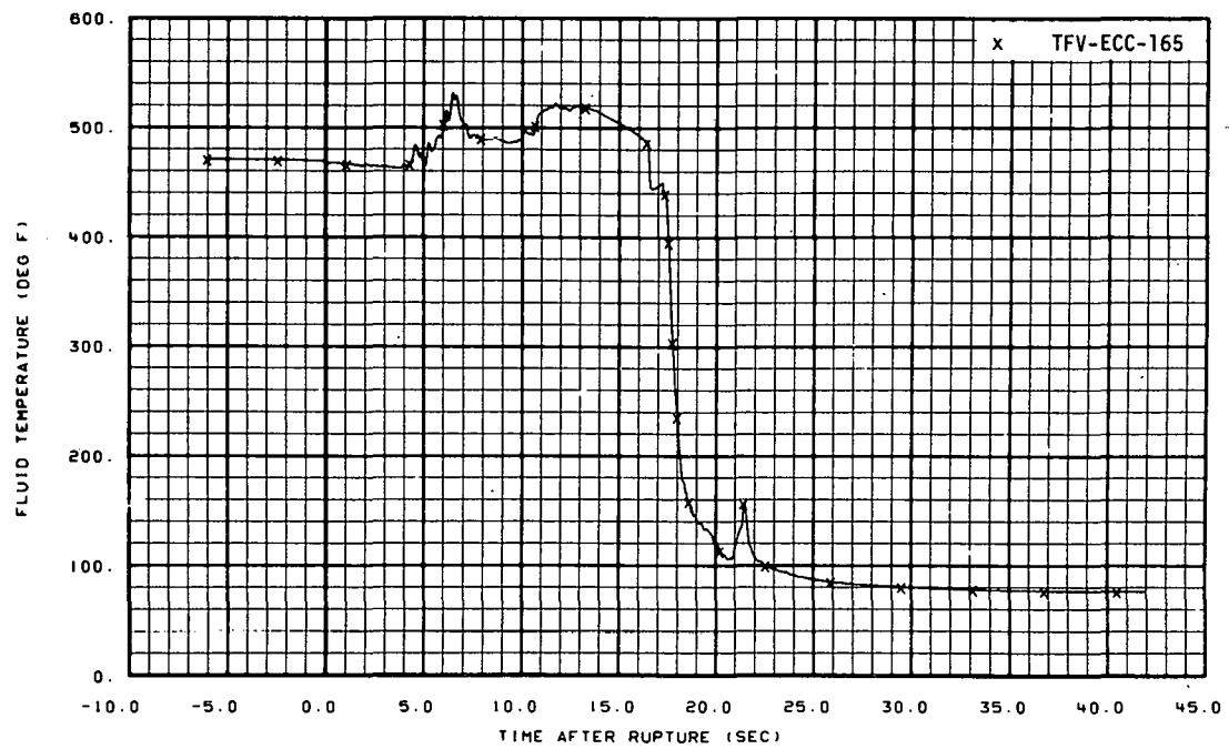
Fig. 32 Fluid temperature in lower plenum (TFV-ECC-165), from -6 to 42 seconds.
