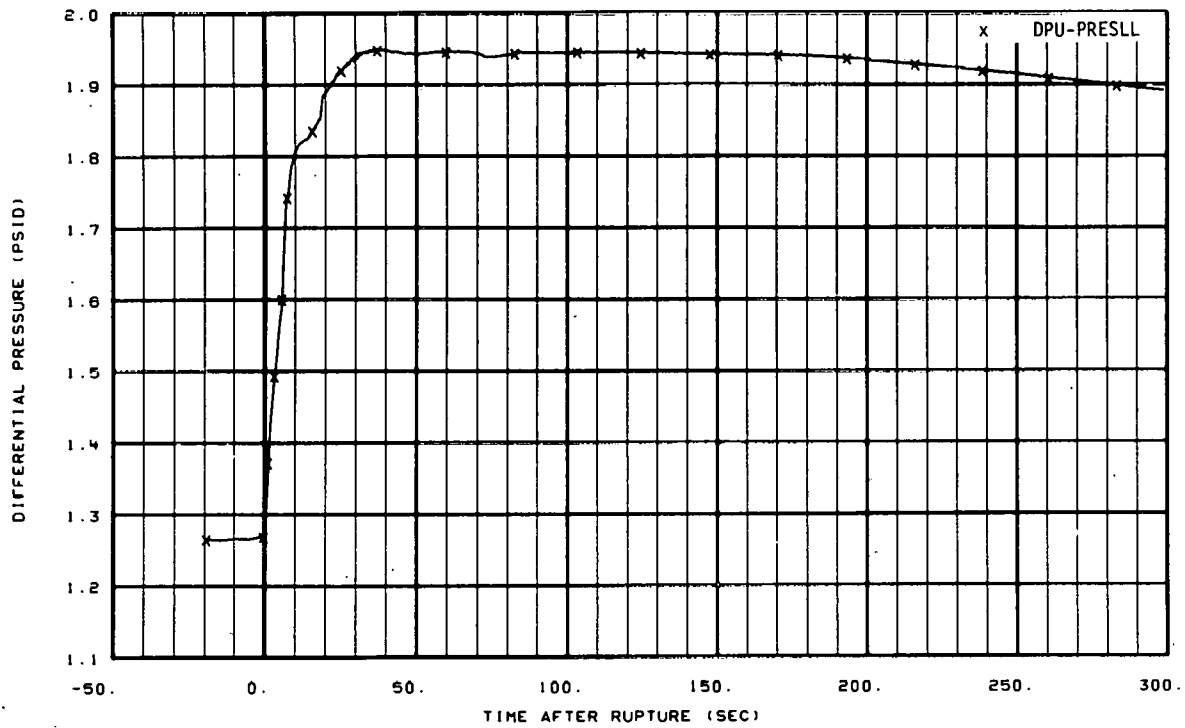
Fig. 165 Differential pressure in intact loop (DPU-PRESLL), from -20 to 300 seconds.
