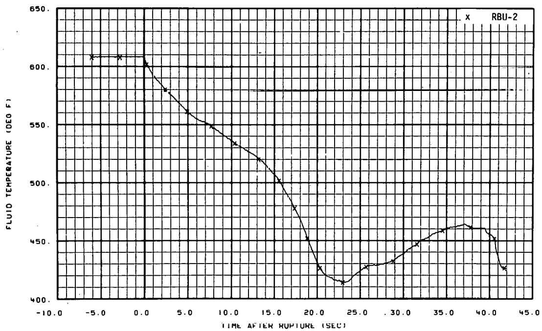
Fig. 10 Fluid temperature in intact loop hot leg (RBU-2), from -6 to 42 seconds.
