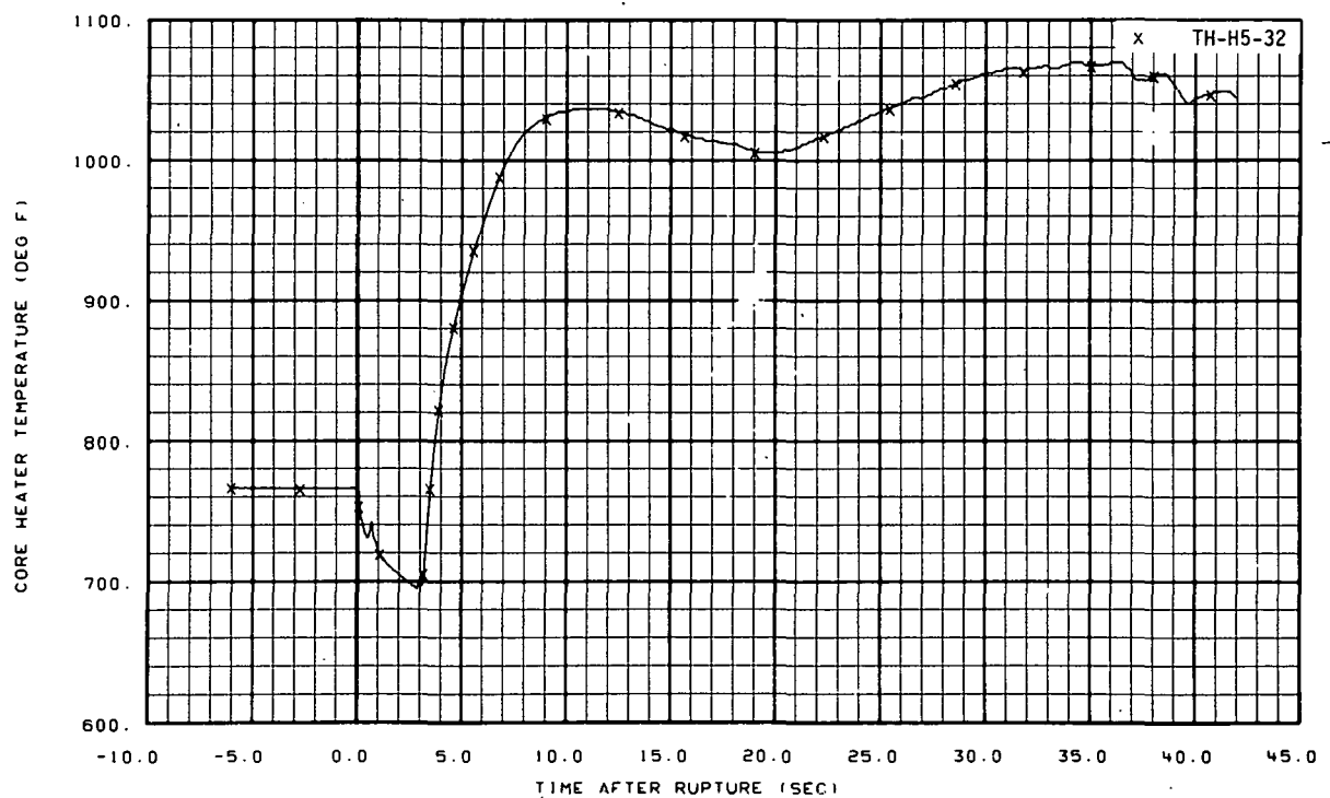
Fig. 124 Core heater temperature, Rod H-5 (TH-H5-32), from -6 to 42 seconds.
