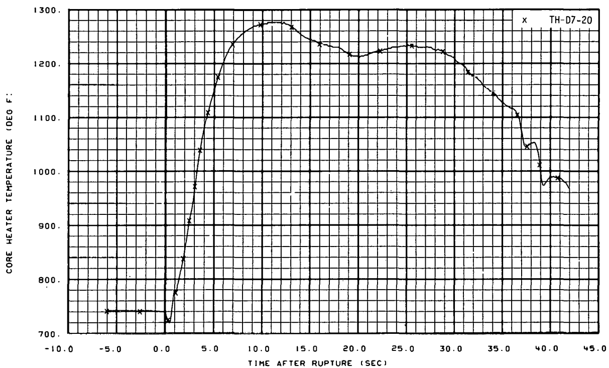
Fig. 94 Core heater temperature, Rod D-7 (TH-D7-20), from -6 to 42 seconds.
