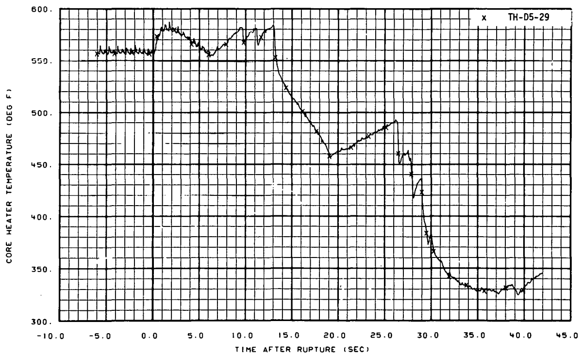
Fig. 60 Core heater temperature, Rod D-5 (TH-D5-29), from -6 to 42 seconds.
