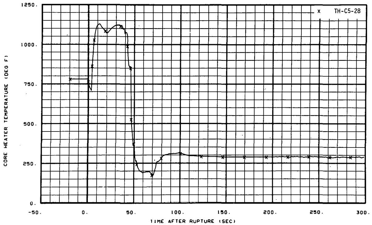
Fig. 79 Core heater temperature, Rod C-5 (TH-C5-28), from -20 to 300 seconds.
