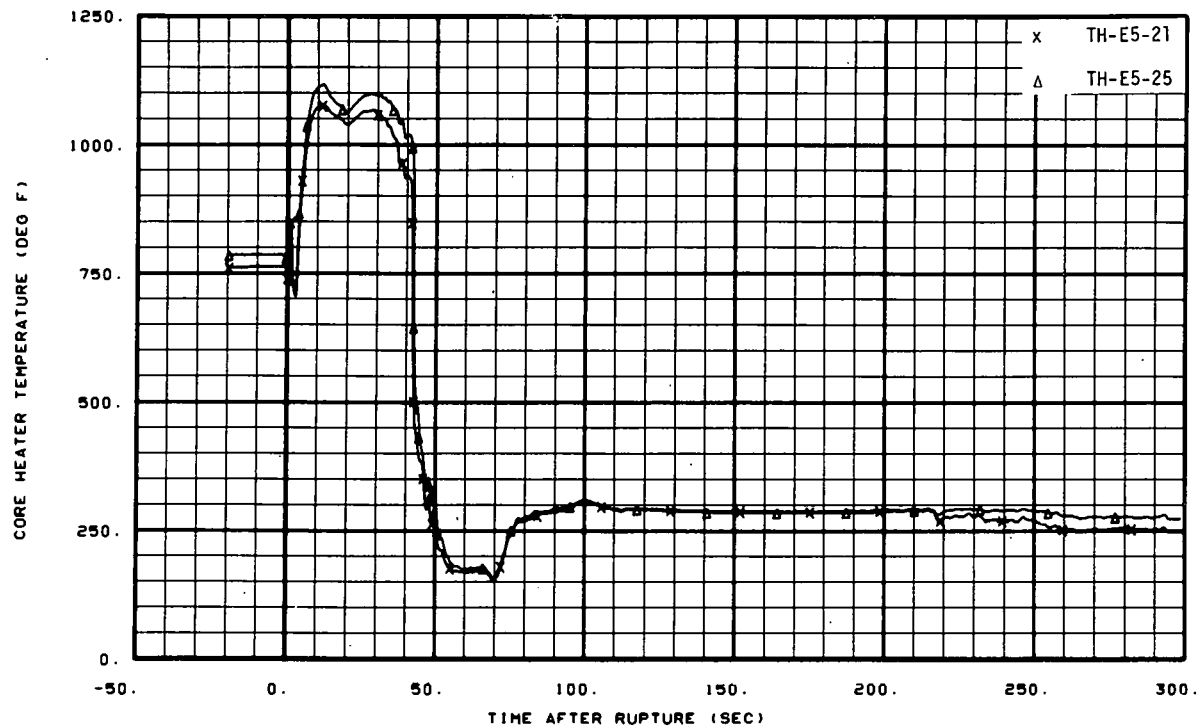
Fig. 63 Core heater temperature, Rod E-5 (TH-E5-21 and TH-E5-25), from -20 to 300 seconds.
