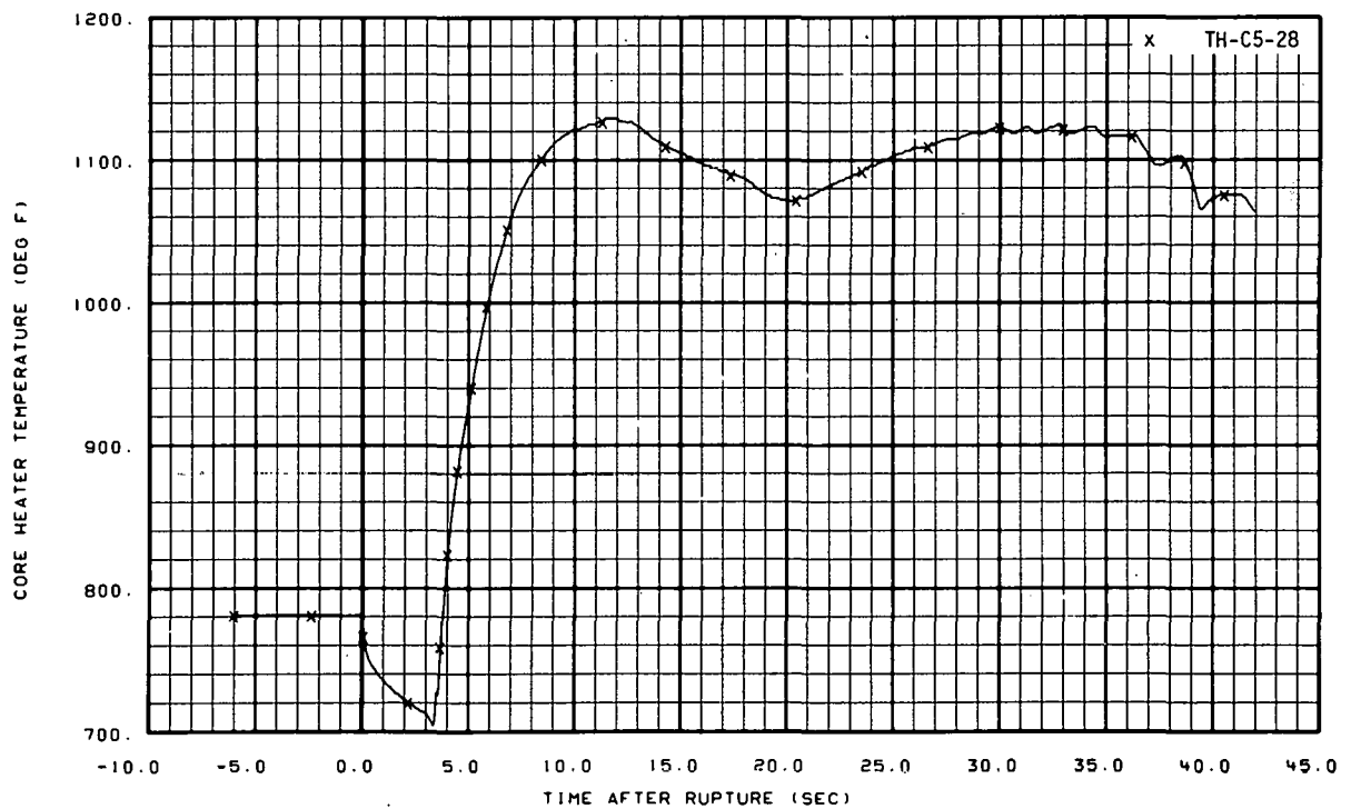
Fig. 80 Core heater temperature, Rod C-5 (TH-C5-28), from -6 to 42 seconds.
