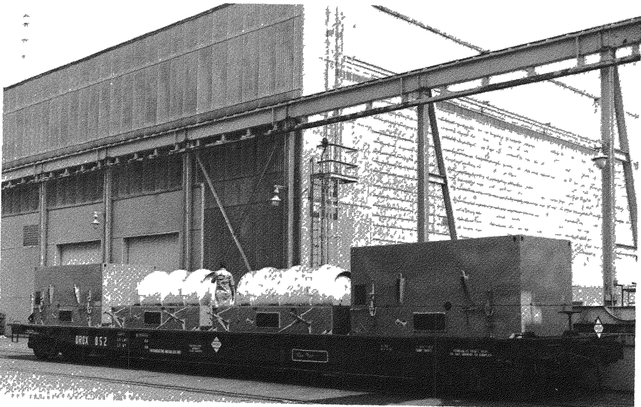
Figure 12 FOUR 10-TON CYLINDERS IN PROTECTIVE OVERPACKS
