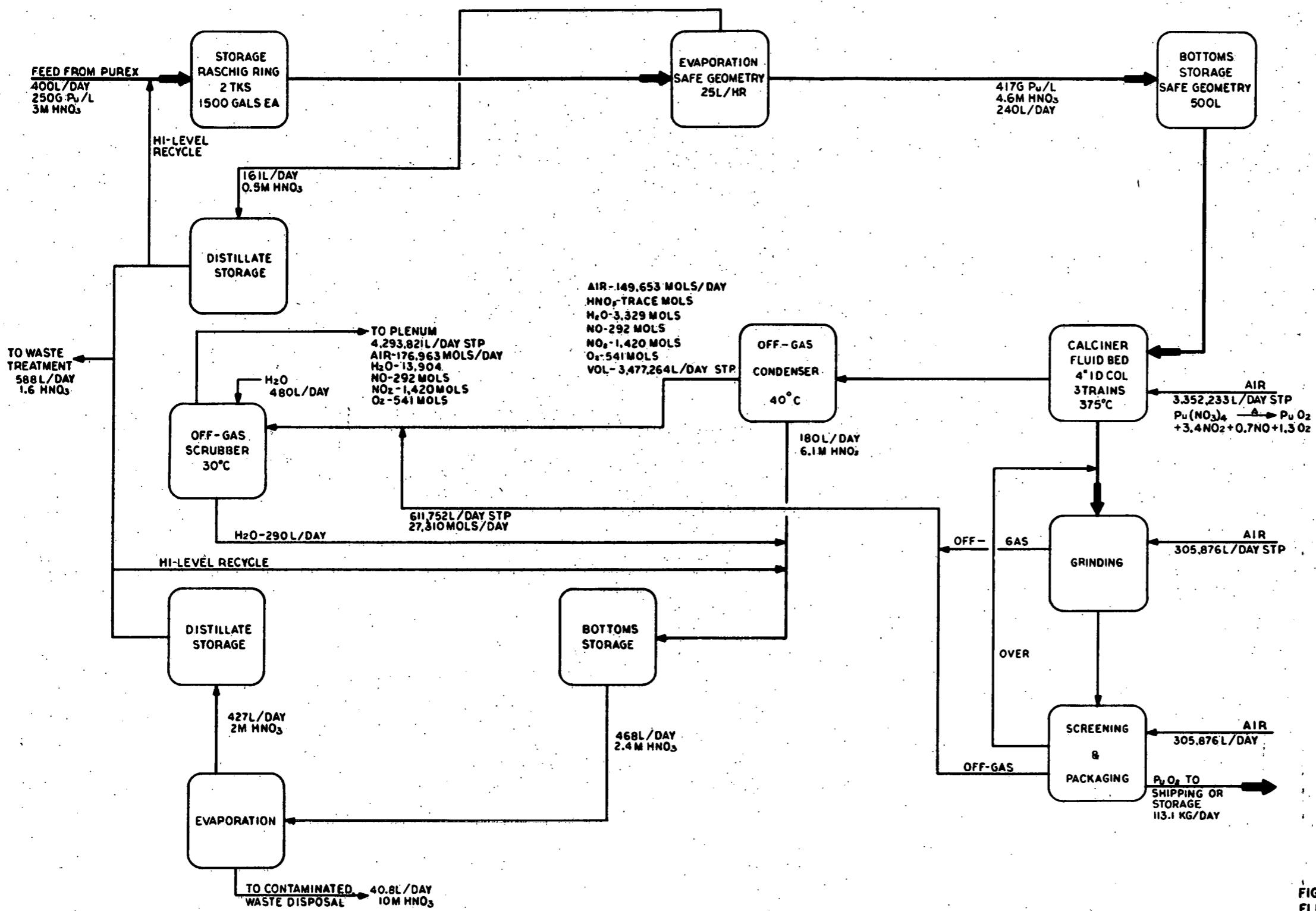
**FIGURE 1. BLOCK FLOW DIAGRAM,
