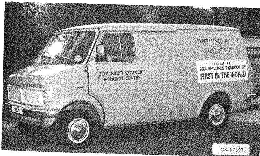
Figure 6. - Na-S battery powered van.
