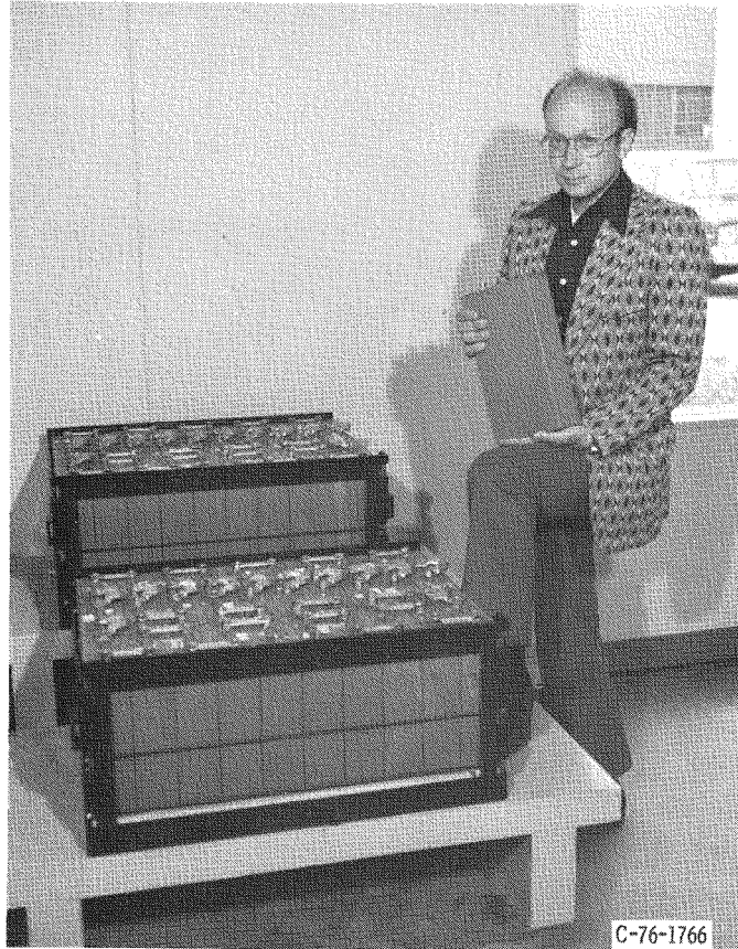
Figure 2. - Nickel-zinc vehicle battery.
