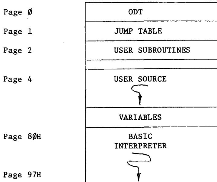
The subroutine table contains 3-byte entries for each subroutine. The table is located at the address specified in the JUMP-TABLE for SUBAD. (Page 1, Location 2)
