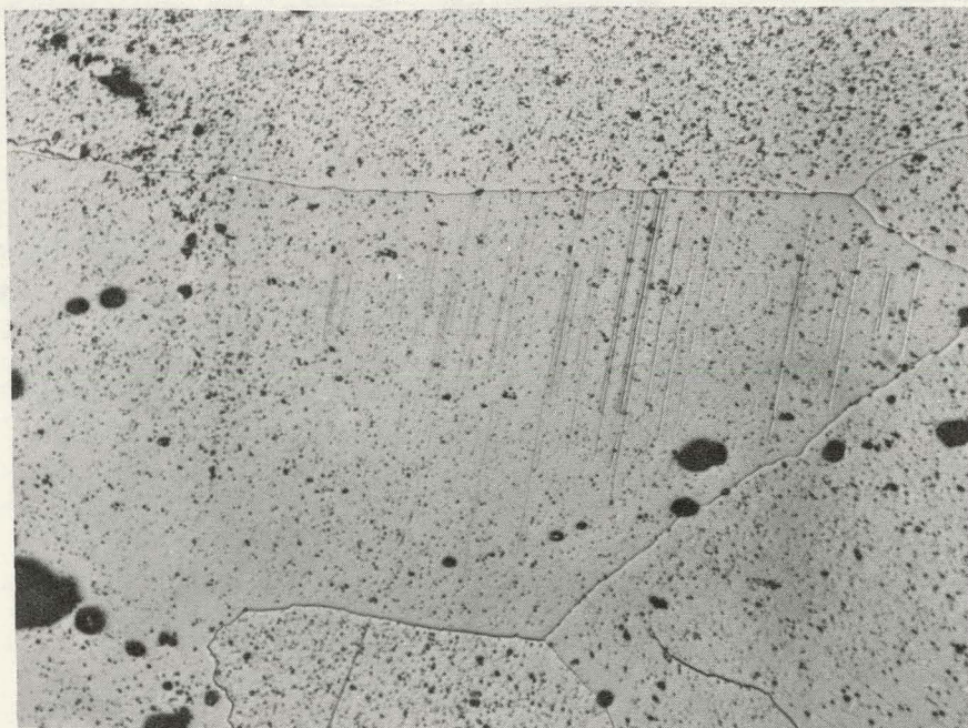
29c Photomicrograph Showing Stress Twins in Grain Exhibiting Exaggerated Growth. Also Note Large Amount of Intragranular Porosity.
