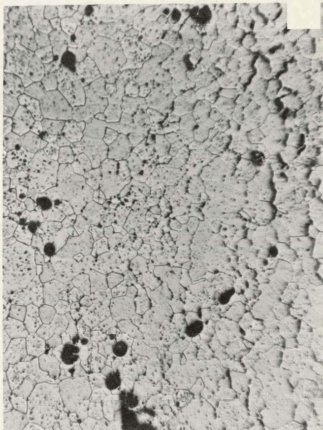
29b Photomicrograph of an Area Near the Pellet Center Showing Grain Boundary Separation (Right Hand Side of Photograph)
