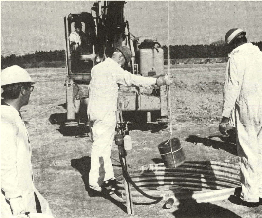
Figure 3. PITC specimen being lowered into lysimeter.
