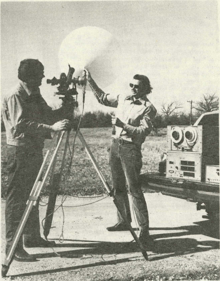
FIGURE 4—MAP3S researchers from Argonne National Laboratory prepare to release and track a small balloon that contains a miniature instrument for measuring temperature. Optical tracking provides information on wind and height, thus adding to the data available (ANL photo).
