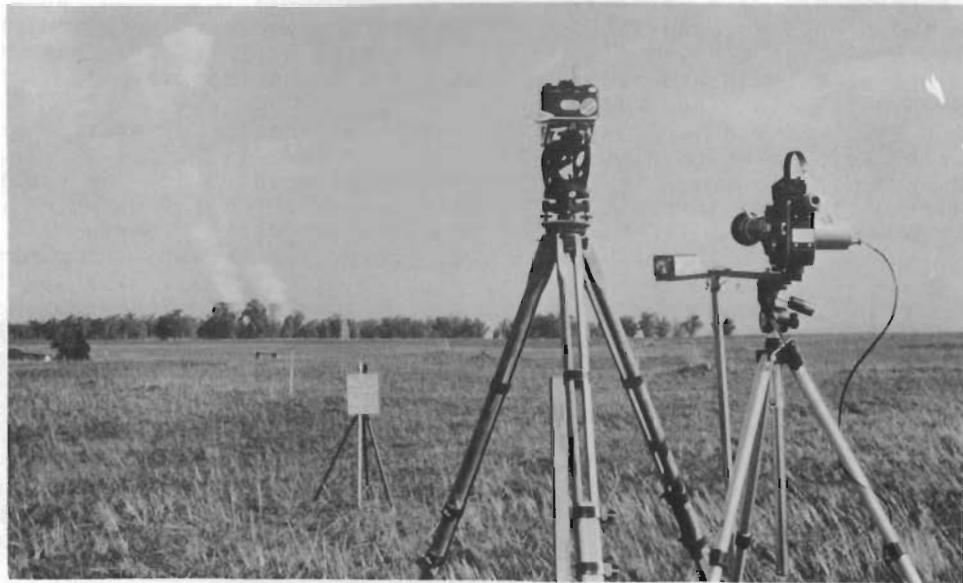
FIGURE 2. Topcon 35 mm Camera on Transit, and 16 mm Bolex Movie Camera in Normal Operating Mode
