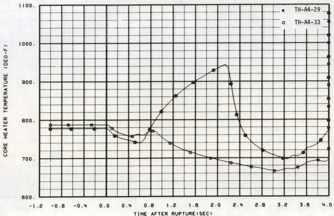
Fig. 53 Cladding temperature response at 29- and 33-inch elevations on Rod A4 - Test S-02-7.
