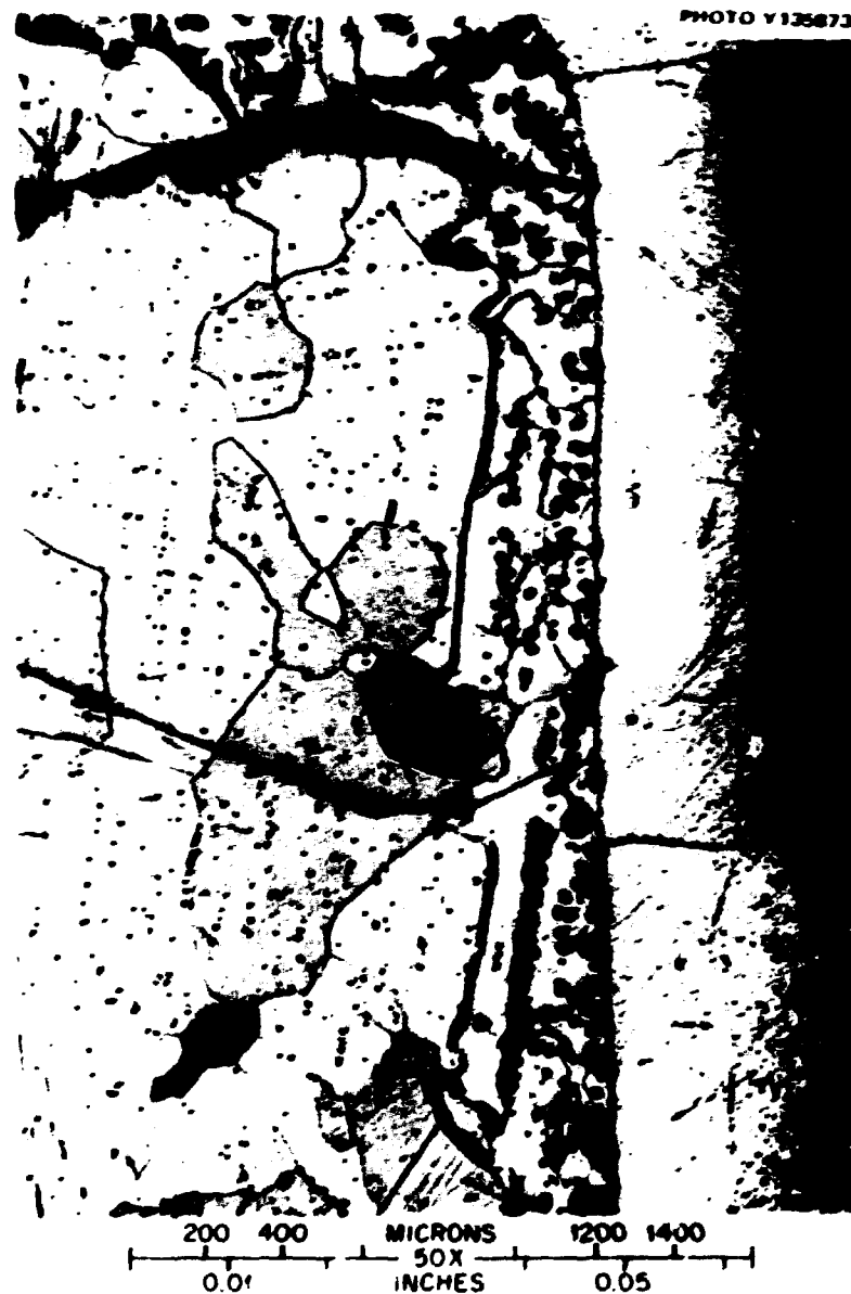
Fig. 5.2. Cross section of a thermally equilibrated niobium plus tin sample. Etched, 50X.
