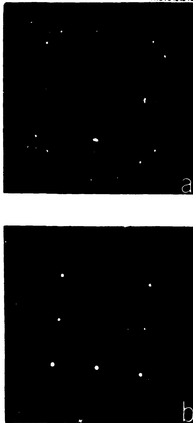
Fig. 2.10. LEED patterns from (001) gold surfaces: (a) clean reordered ( 5 \times 20 ) structure and (b) normal ( 1 \times 1 ) structure produced by O_2^+ ion bombardment. Primary beam energies (a) 64 eV and (b) 107 eV
