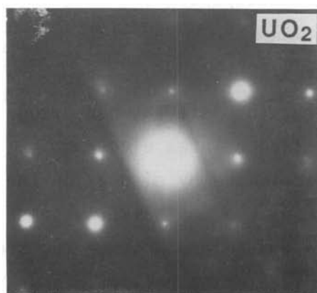
FIGURE 4.3. \text{U}_4\text{O}_9 Formation Along Grain Boundaries in Oxidized Monticello BWR Fuel ( 135^\circ\text{C} oxidation; average \text{O}/\text{M} = 2.016 ): a) Transmission Electron Micrograph; b) Selected-Area Diffraction Pattern from \text{UO}_2 Region; c) Selected-Area Diffraction Pattern from \text{U}_4\text{O}_9 , Showing Extra, Diffuse-Scattering Reflections
