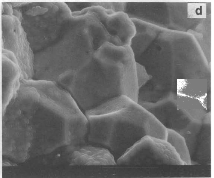
FIGURE 4.12. Powder Particles from Oxidation Tests; SEM Micrographs: a) Sample 87-03, Oxidized at 135°C, Average O/M - 2.007; b) Higher Magnification View of (a); c) Sample 86-38, Oxidized at 150°C, Average O/M - 2.15; d) Higher Magnification View of (c)
