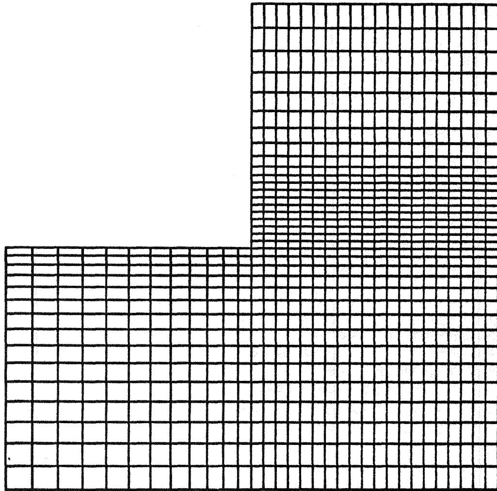
Figure 2. Sample MERCURY output showing a coaxial conducting structure overlaid on the mesh
