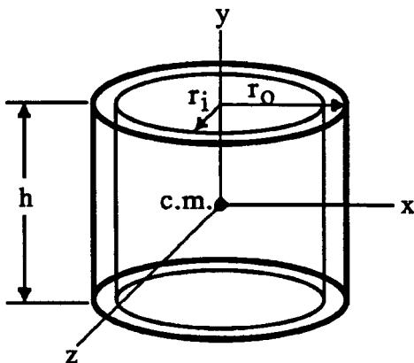
$$I_{xx} = I_{zz} = \frac{\rho \pi r_o^2 h}{12} (3r_o^2 + h^2) - \frac{\rho \pi r_i^2 h}{12} (3r_i^2 + h^2)$$
