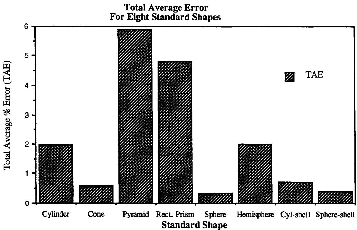
From the above graph, it is seen that ANVIL 5000's computed mass properties are the most accurate for a sphere and least accurate for a pyramid. As would be expected, ANVIL 5000's mass properties computations are most accurate for shapes with rotational symmetry.
